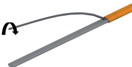
Push the green/yellow heat shrink tube (length: 4 ¾" (120 mm); diameter: ¼" (6 mm) onto the twisted grounding braid. **9**
