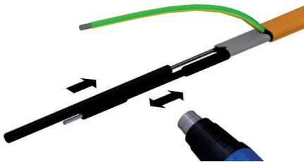
Push the outer heat shrink tube (length: 1" (25 mm); diameter: ½" (12 mm)) over the end of the trace heater.
