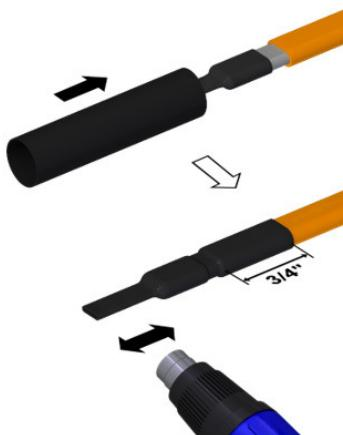
Installation Instruction Power connection kit - Cable to Junction Box with  $\frac{1}{2}$ " NPT cable gland
