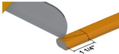
Remove the exposed grounding braid. Make sure that the insulation jacket is not damaged.
