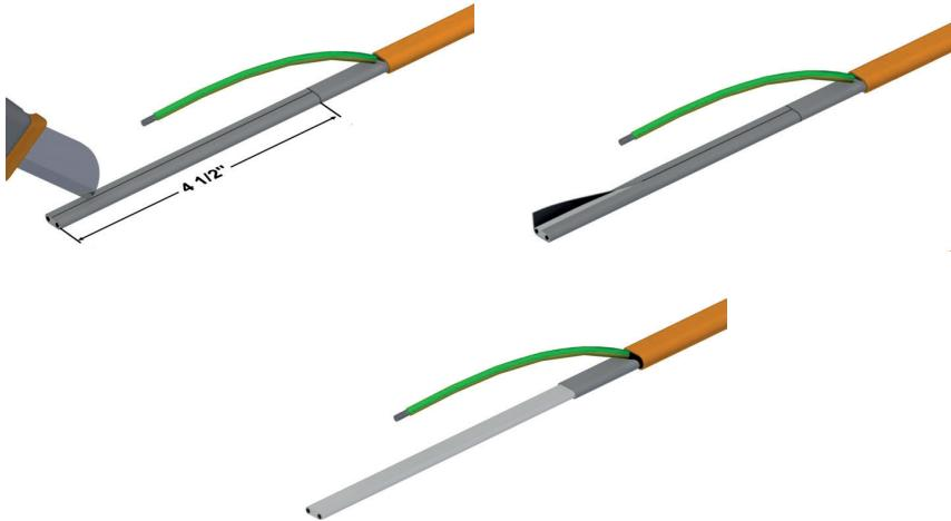
Make a small cut over and under each bus wire. Take care not to damage the bus wires.
