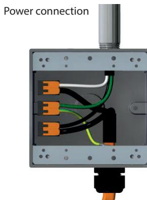
Mount the cover of the junction box according to the manufacturer's installation instructions.
