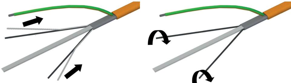
Remove the remaining heating matrix. Take care not to damage the bus wires.
