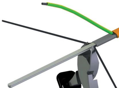
Carefully cut in a triangle (1/8" (5 mm)) between the bus wires. Take care not to damage the bus wires.
