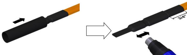
Fold over the overlapping end of the heat shrink tube  $\frac{3}{8}$ " (10 mm).
