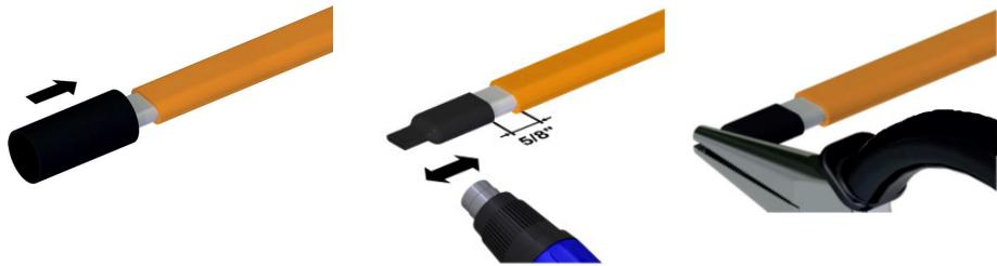
Now, put the outer heat shrink tube (length:  $2\frac{3}{4}$ " (70 mm); diameter:  $\frac{3}{4}$ " (19 mm)) over the end of the trace heater.
