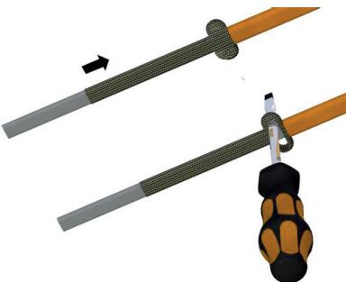
Bend the trace heater and pull the heating matrix out of the grounding braid. **7**
