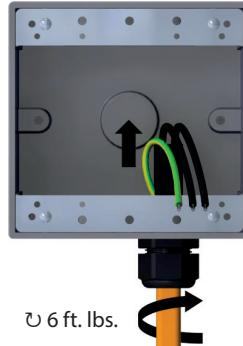
For powered splice and powered T connection kits repeat steps 3 to 16 to prepare the remaining trace heaters, introduce them into the junction box and tighten the gland.
