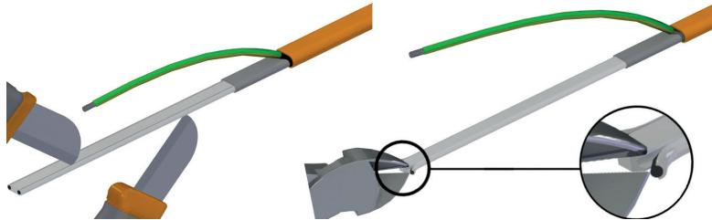
Pull off the bus wires while holding the heating matrix.
