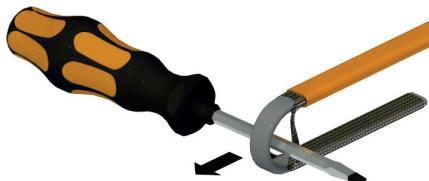
Twist the grounding braid in order to form a wire. **8**
