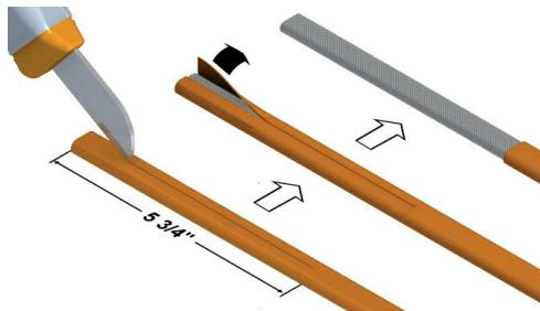
Push the grounding braid back. Use the screwdriver to form an eyelet. Be careful not to damage the internal insulation jacket **6**
