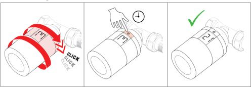
Screw the Danfoss  $Eco^{TM}$  onto the mounted adapter until a click sound appears. Once the thermostat is tightened properly, then adjust the display to your preferred display orientation. A large M is flashing in the display to indicate that Installation Mode is activated. Press and hold the button  $\bigcirc$  for 3 seconds.
