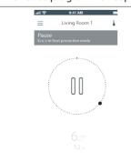
When Danfoss Eco<sup>™</sup> is turned down to Min level manually, a notification banner is shown, and center icon switches to 'Pause'.
