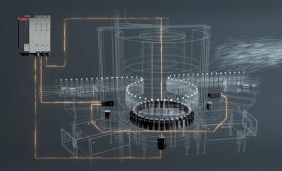
The decentral servo drives ISD® 510 and DSD 510 are available with enclosures rated up to IP67.
