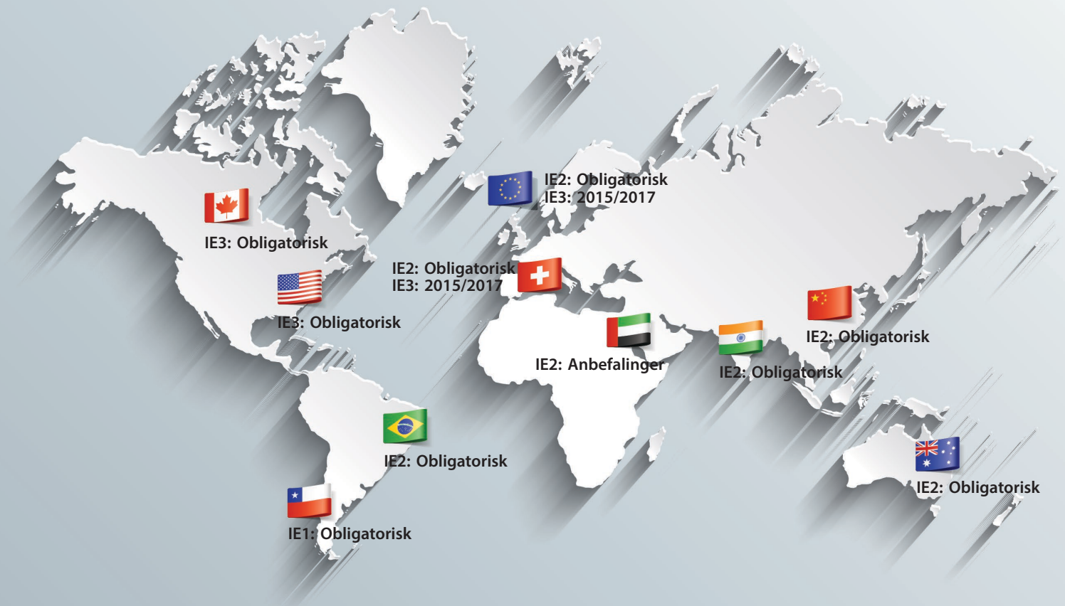
This selection of currently applicable and upcoming minimum requirements shows that the efficiency of electric motors is a worldwide issue.
