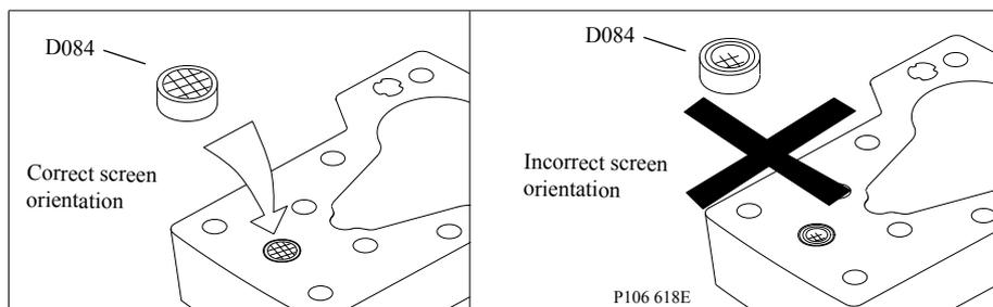
3. If previously removed, install orifices using a 3 mm internal hex wrench and torque to 2.5 N·m [1.8 lbf·ft].
