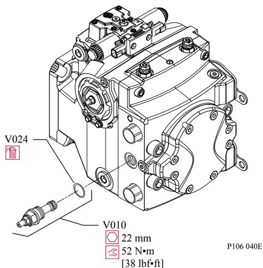
1. Using a 22 mm wrench, remove the charge pressure relief valve (V010).
