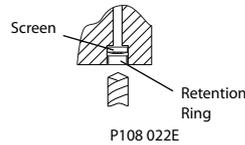
Note screen orientation for reassembly.
