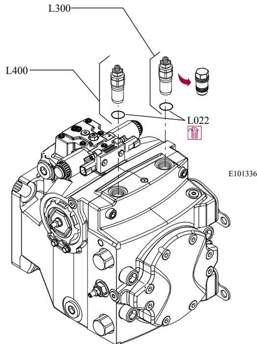
1. Using a 22 mm or 24 mm wrench, remove the pressure limiter valve (L100), and discard the O-ring.
