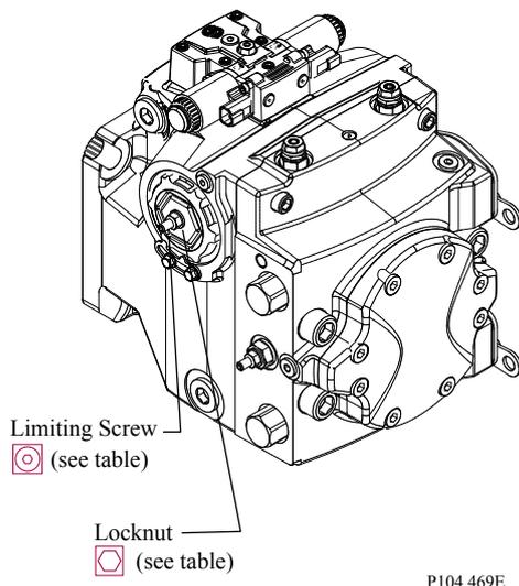
1. Loosen the locknut.
