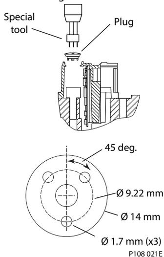
3. Push down on plug and turn 45 degrees counterclockwise.
