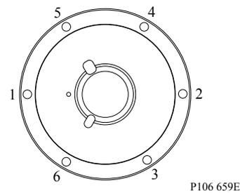
11. Ensure proper torque on aux. pad screws (K400), and if necessary, replace screws.
