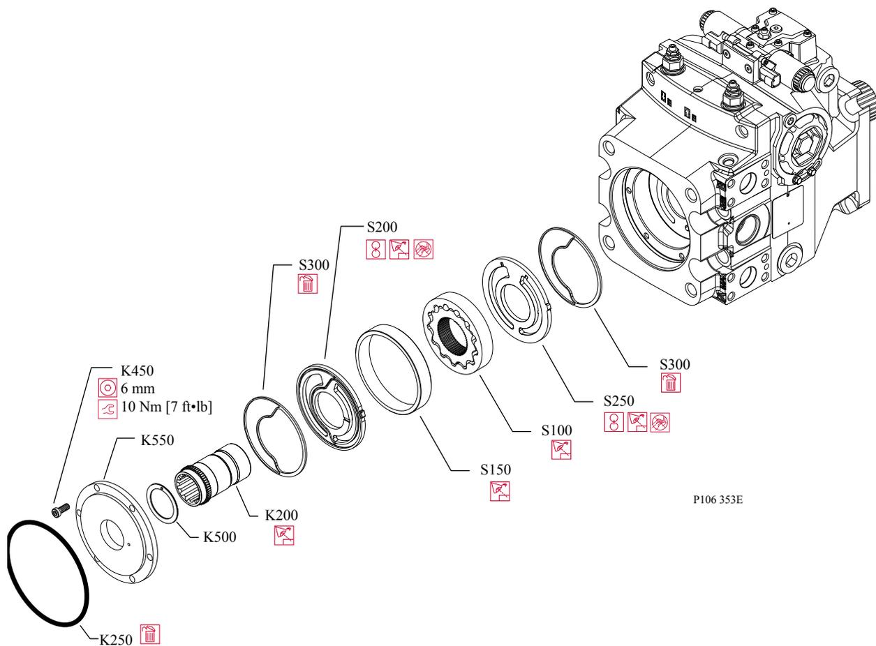
1. Remove auxilliary pump and O-ring (K250), and discard O-ring.
