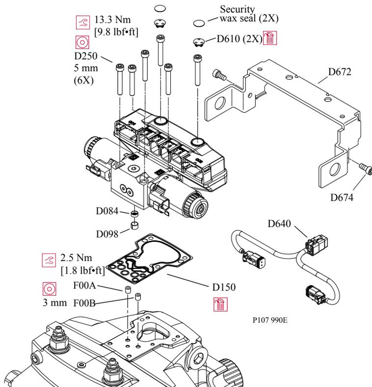
1. Disconnect and remove wiring (D640).
