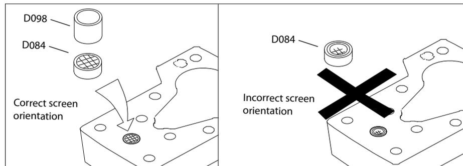
3. If previously removed, install orifices using a 3 mm internal hex wrench and torque to 2.5 N·m [1.8 lbf·ft].
