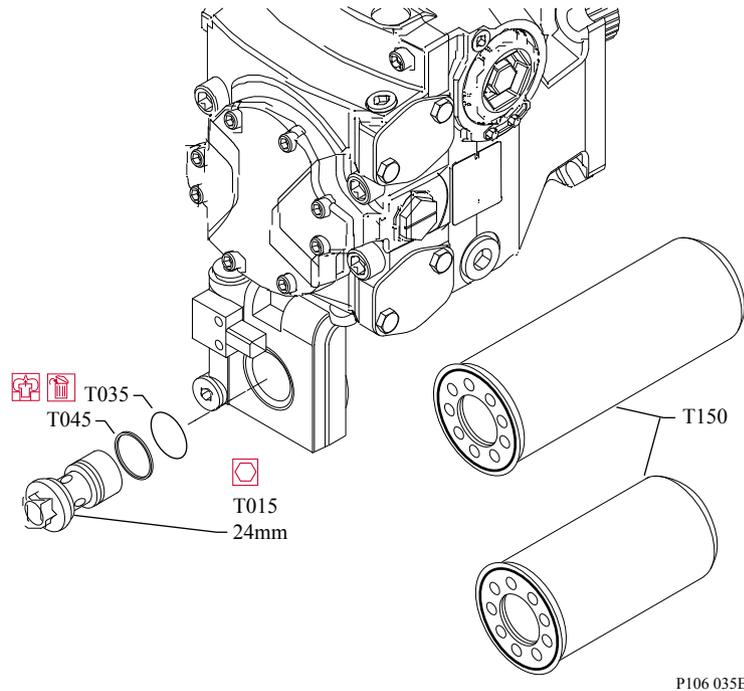
1. With the prime mover off, hold the filter (T150) in place, and remove the plug (T015) using a 24 mm wrench.
