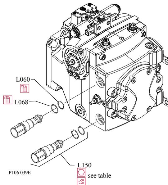
1. Using a hex wrench wrench shown in the table below, remove the HPRVs (L150).
