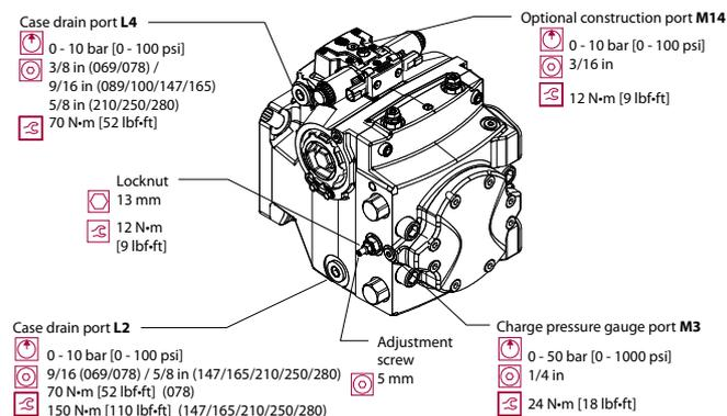
1. Install a 50 bar [1000 psi] pressure gauge in charge pressure gauge port M3.
