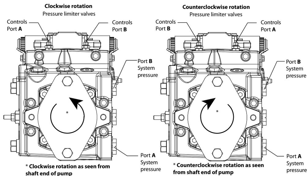
If you change pressure limiter settings, you must also change the HPRV valve to maintain proper PL function. Refer to table below for corresponding settings.
