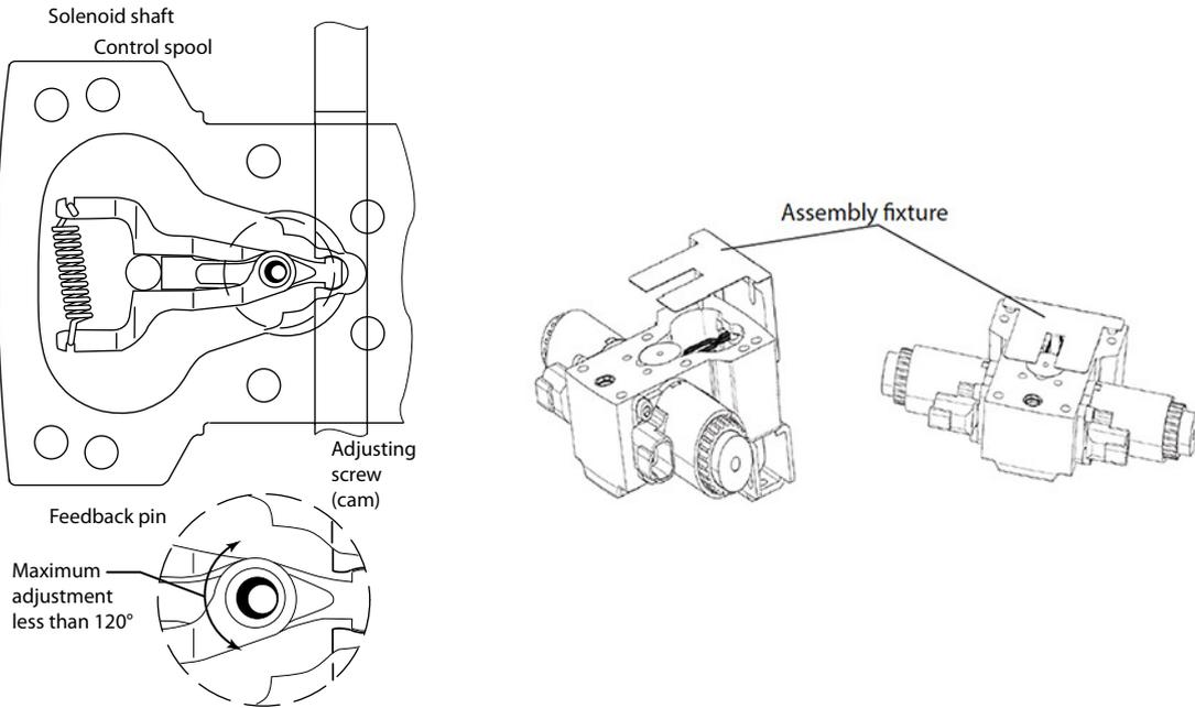
Remove plug (D065) and verify the swashplate feedback pin is properly positioned between control feedback arms.
