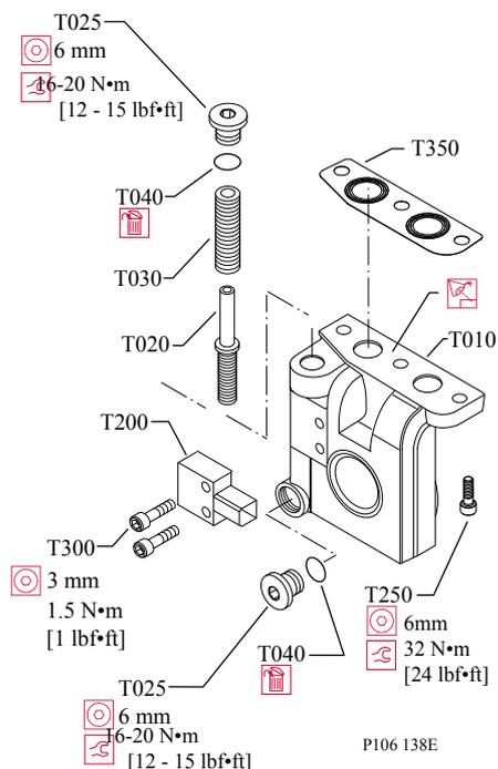
1. Remove three screws (T250) using a 6mm internal hex wrench.
