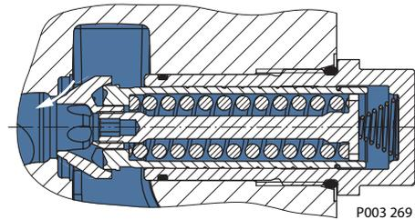
**Charge Pressure Relief Valve (CPRV)**
