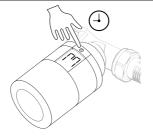
Press and hold until large fill flashes. This indicates you are in mounting mode 2.
