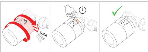
Screw the Danfoss  $Eco^{TM}$  onto the mounted adapter until a click sound is heard. Once the thermostat is tightened properly, then adjust the display to your preferred display orientation. A large  $\mathfrak{M}$  is flashing in the display to indicate that Installation Mode is activated. Press and hold the button  $\mathfrak{A}$  for 3 seconds.
