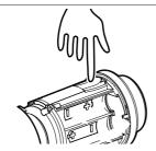
Press firmly on the tab and unscrew the thermostat from the adapter.
