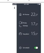
Scroll on temperatures to set your preferred temperatures. The Danfoss Eco™ can be set from 5°C to 28°C. Danfoss recommend a difference between 'At Home' temperature and 'Away/Asleep' that does not exceed 4 degrees.
