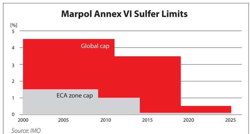
Figure 1: MARPOL Annex VI sulfur limits
