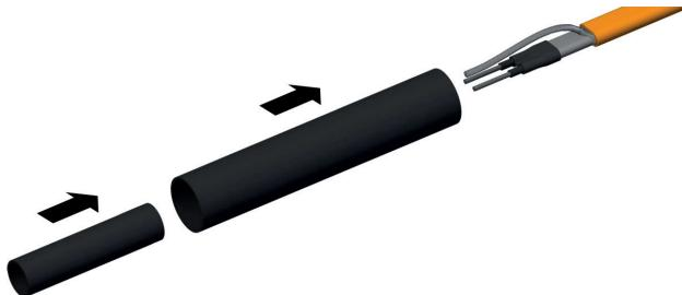
Slide a ferrule (no. 3) onto both of the bus wires.
