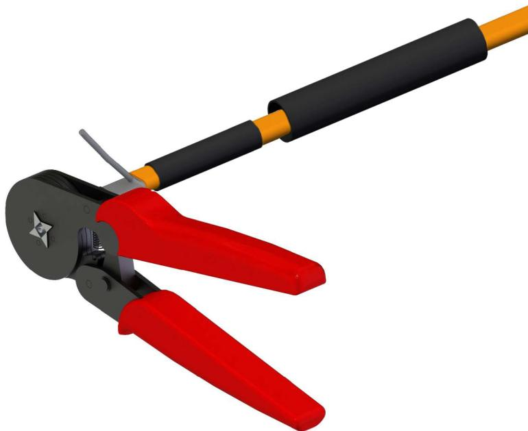
Slide the bus wire splice lugs (no. 1) all the way onto the bus wires and crimp them on.
