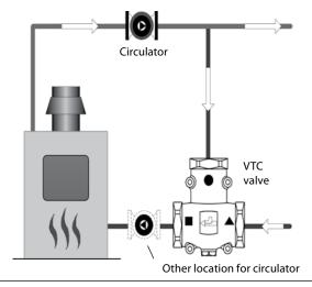
When the VTC is piped on the supply side out from the heat source, the valve will begin to allow water out to the system when the temperature of the fluid meets the temperature of the inserted thermostat element.
