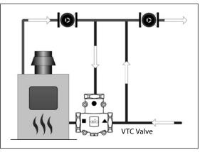
Because gravity conversion systems contain an enormous volume of water, the water returning to the heat source could be significantly cooler, leading to condensation and a shorter life for the heat source. Adding a thermic valve to the system will prevent the boiler from sustained operation at temperatures below the dew point of their flue gases.
