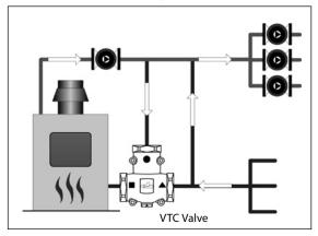
Where a high mass non condensing heat source is matched with a large low temperature system, a situation could occur where the heat source is unable to keep up with the rate of demand from the system. The use of the thermic valve provides the opportunity for the heat source to catch-up.
