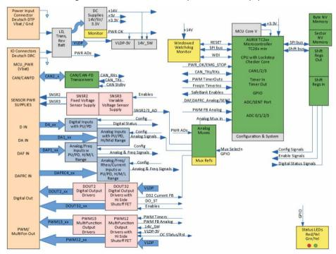
The MCU will execute the Modular Safety Kernel (MSK). The inputs will be read and provided to the application. The application processes this information and will set the outputs to the desired values. The setting of the outputs is done from the MSK.
