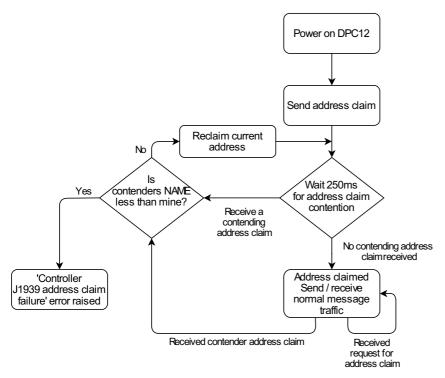
For the full address claim procedure refer to SAE J1939 standard or contact your Danfoss representative.
