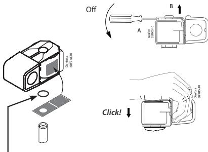
Recommended to reduce vibrations, not required for sealing.
