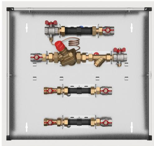
Danfoss Metering Unit is a heating and cooling unit, which can be used for metering, balancing, and controlling of individual apartments in centralized heating and domestic hot water systems. The modular version consists of different articles that are fully compatible and can be easily mounted to all pipe directions. In PV-PM-BD sets are already pre-assembled.
