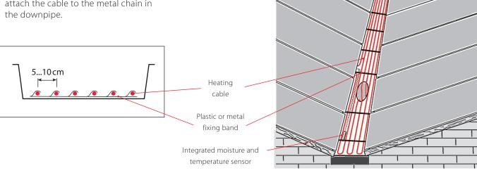
Gutter valley heating cable installation
