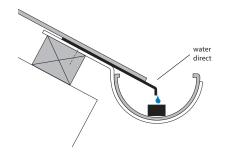
Steep roofs facing south may be exposed to the strong sunlight and as a result fast water dry out. In such cases it may be required to install some additional means to direct water towards a moisture detecting sensor.
