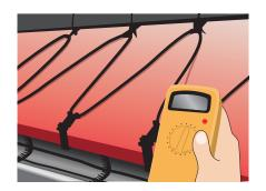
Install the cable(s) on the roof, in gutters and downpipes. Check once again and compare the insulation resistance and Ohm rating for constant wattage cables.
