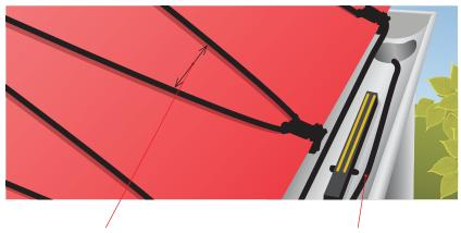
**C-C** – Average cable distance in cm in gutter valleys and on roof areas
