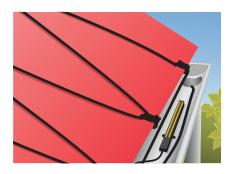
Install ECtemp 850 external sensor, if any, in the gutter according to the sensor manual.
