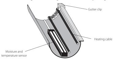
The heating system will be placed in a standard plastic gutter length 37,5 m combined with two drainpipes, with a length of 15 m each. These pipes enter the system sewerage placed approx. 1 m beneath the ground surface.
