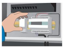
Check once again and compare the insulation resistance and Ohm rating for cables. Install ECtemp thermostat and connect cables to the connection boxes and to the switchboard.
