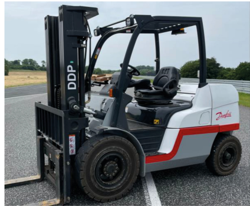
Figure 3 - Converted Digital Displacement Forklift
