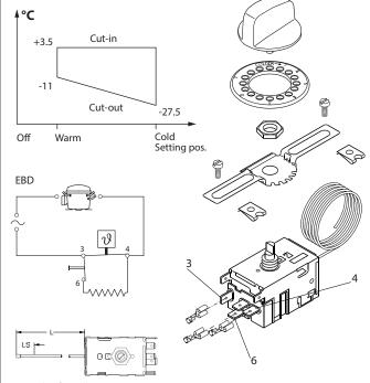
Length of capillary (mm): L = 1600 + 50/-0Min. sensor length mounted on evaporator (mm): LS = 125(Used as airsensor min.  $2 \times LS$ )
