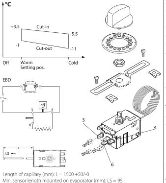
(Used as airsensor min. 2 x LS)
