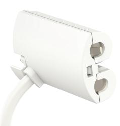
Danfoss Ally<sup>™</sup> Power Module 24V is an accessory that connects the electronic radiator thermostat to an existing power system in the building and enables the device to work without batteries. The power output must be a 24 V supply from a safe source with a class II insulation level (Power supply with built-in double or reinforced insulation level between the supply voltage and safe voltage).
