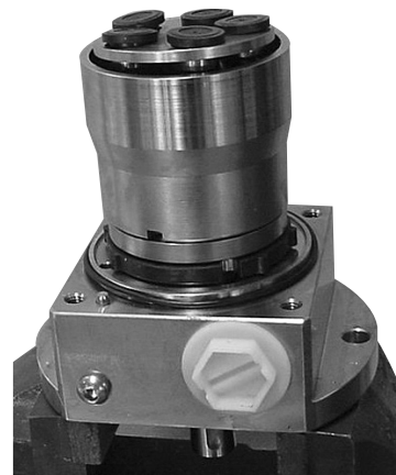
11. All pistons inserted.
