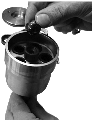
10.2.a. Remove the retainer guide.
