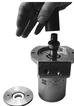
24. Use the shaft seal tool when pressing the shaft seal downwards.
