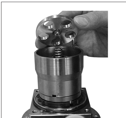
9.1.c. Mount the retainer plate.
