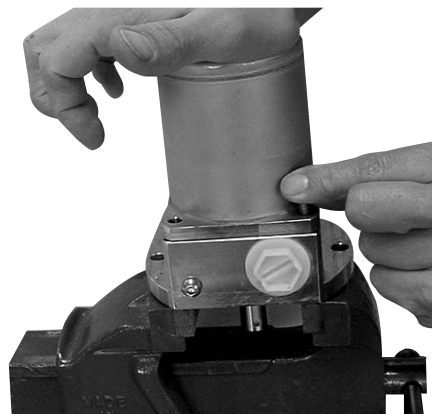
16. Press the housing down by hand and insert the screws.
