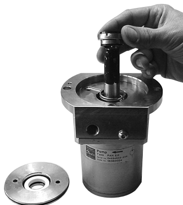
23. Wet the shaft seal and slide it over the bush.
