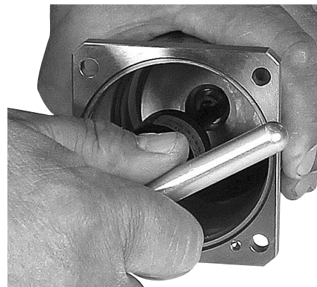
14. Tighten to a torque of 10 \pm 1 Nm.
