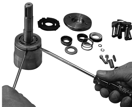
11. Loosen the valve plate using two screwdrivers. Place one of the screwdrivers in the slot of the valve plate.
