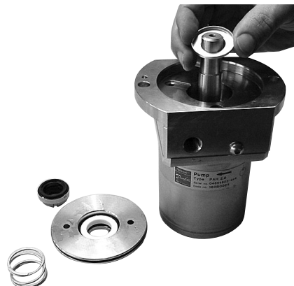
20. Mount the washer with the edge pointing upwards.
