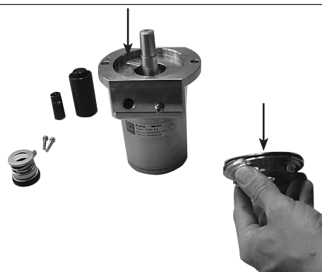
18. Mount the two O-rings in the flange and the O-ring on the front cover.
