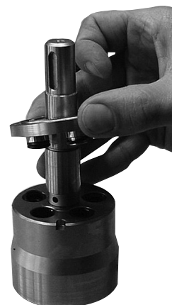
12. Remove the valve plate.
