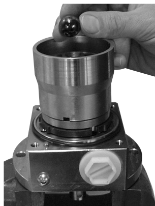
9.2.c. Mount the retainer guide on the spring guide.
