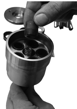
10.2.b. Remove the spring guide.
