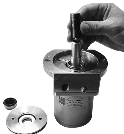
22. Fit the hollow bush onto the shaft.
