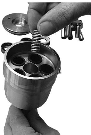
10.2.c. Remove the spring.
