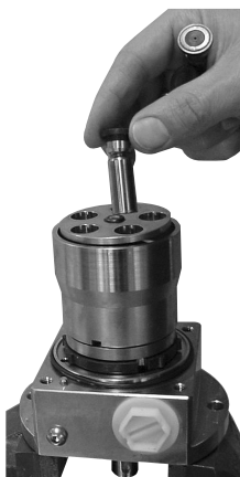
10. Insert the pistons.
