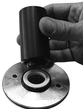
19. Wet the shaft seal with water and mount it in the front cover. Ensure that it is pressed to the bottom.
