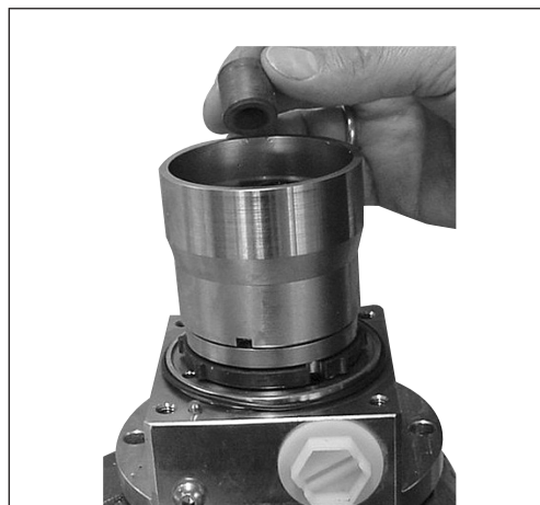
9.2.b. Mount the spring guide.
