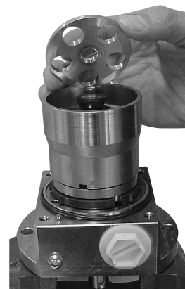
9.2.d. Mount the retainer plate on the retainer guide.
