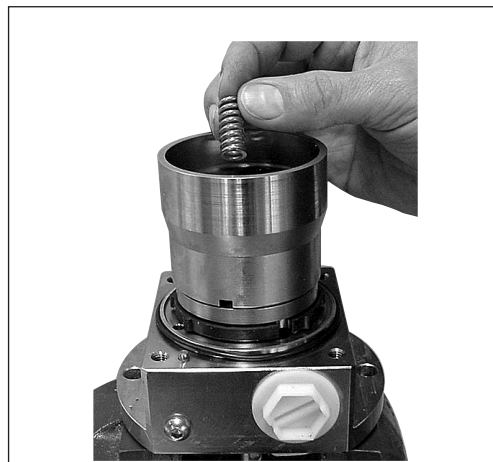
9.1.b. Mount the spring in the centre hole.
