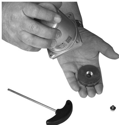
2. Remove swash plate and guide pin.
