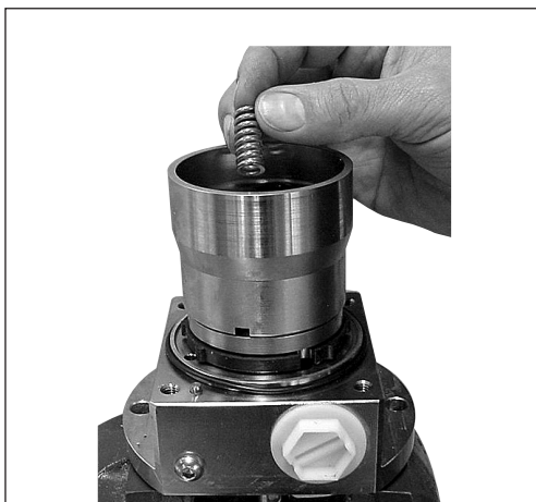
9.2.a. Mount the spring in the centre hole.
