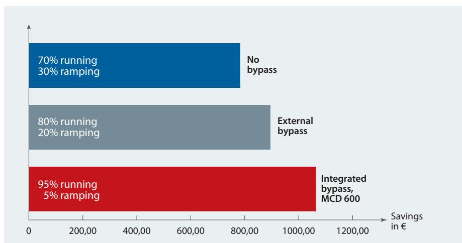
*Cost saving using a bypass, showing the beneficial savings effect of increased running time and reduced ramping time.*
