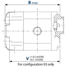
For configuration 06 (SAE A-A) dimension B and V have to be increased 4.5 mm [0.177 in].
