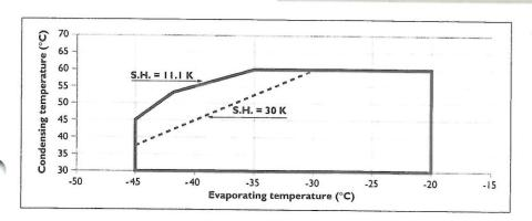
Application Envelope for LTZ compressors with R404A/R507
