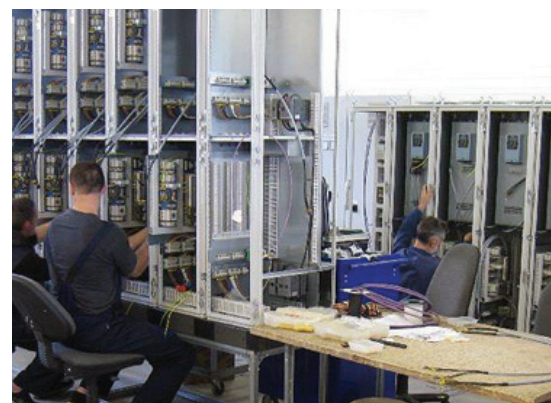
VACON® Active Front-End/common DC bus units being installed in switchgear. Vacon's Active Front-End technology complies with the most stringent harmonic distortion requirements, set by the Norwegian classification body Det Norske Veritas. If required, it also enables the energy generated by winch braking to be fed back into the vessel's electrical network.
