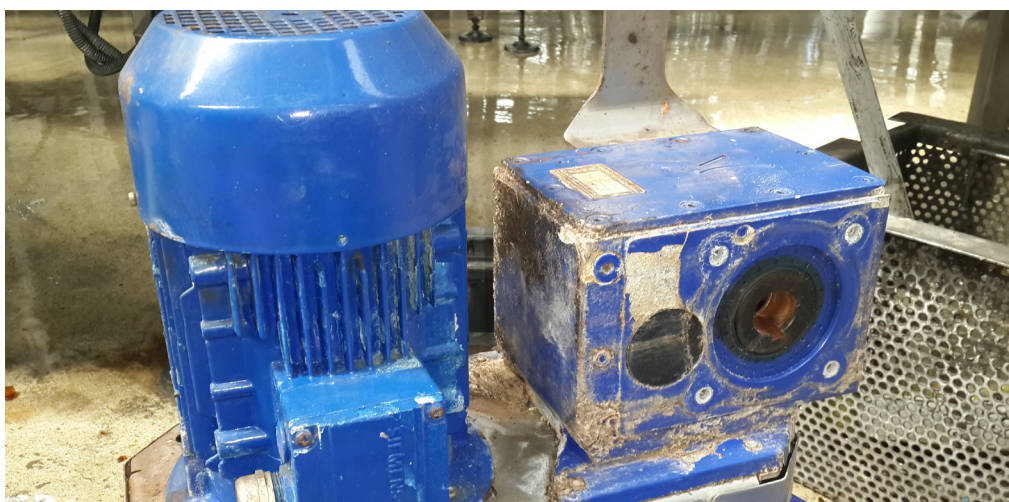
Lower picture: Before the upgrade of the Efes Pilsen Adana plant, this gear motor caused production losses on the bottle-washing line. It needed replacement every year due to corrosion.
