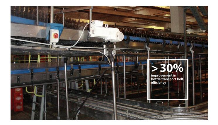
Therefore, a decision was made to upgrade not only the drive that utilizes the VLT® AutomationDrive FC 302, but also the engines, with the VLT® OneGearDrive® permanent magnet gear motors replacing the traditional gear motors that had been installed.
