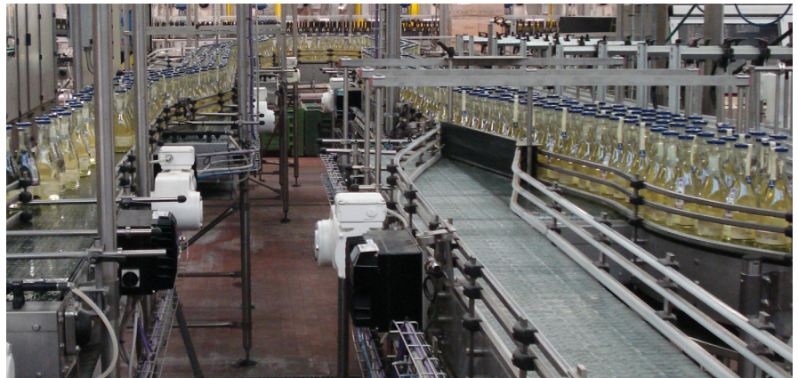
Bottling line with VLT® OneGearDrive® and VLT® Decentral Drive FCD 302 installed directly on the conveyor
