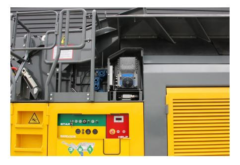
RUBBLE MASTER uses VACON® 100 X drives in their new mobile crusher RM V550GO! to control two unbalanced motors in parallel which run a vibrating conveyor. For RM, the VACON® 100 X provides a customized solution in a standard device, fulfilling all RM's requirements.
