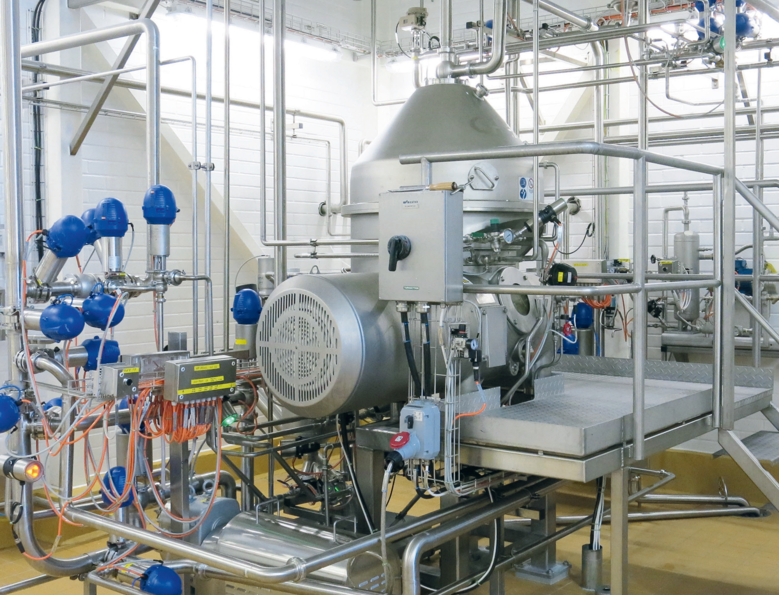
Valio's Seinäjoki plant produces all Valio quarks. A separator is used for producing quark. The pumps and mixers used by the separator are controlled by VACON® 100 AC drives. In recent years, quarks have been the quickest-growing product category in retail sales. Valio was able to quickly double its production at the Seinäjoki plant as butter production had recently moved to new premises.
