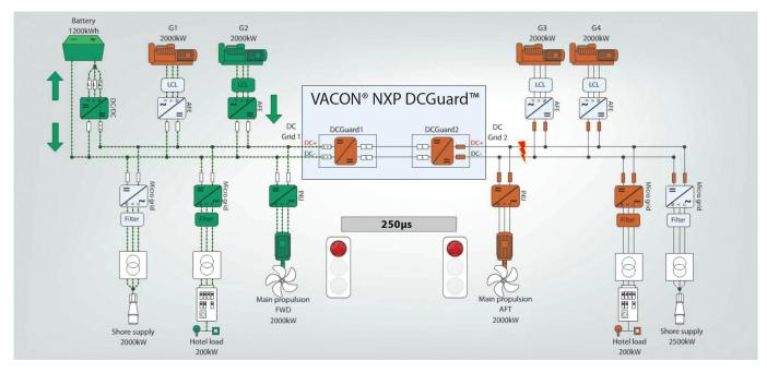
*Figure 5* Short circuit after 200 µs.
