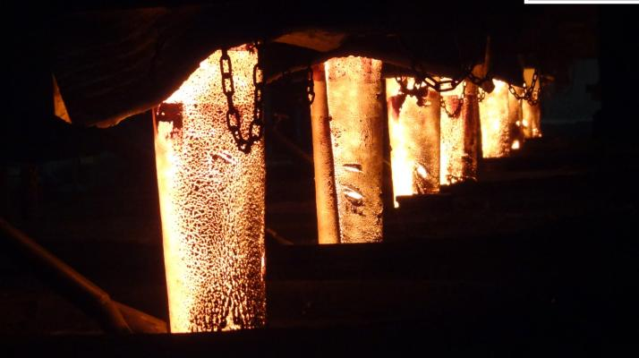
Rarely is reliable uptime so critical, as during continuous casting at a steelworks. To ensure reliable 24/7 operation of continuous casting, system integrator Ingeteam chose VACON® NXP drives to regulate the electromagnetic stirring (EMS) process at the renowned Třinecké železárny a.s., the largest steelworks in the Czech Republic.
