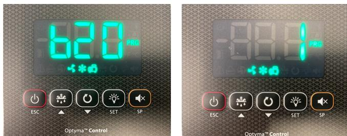
Fig. 6: Parameter “b21” set to 1, for baud rate 19200
