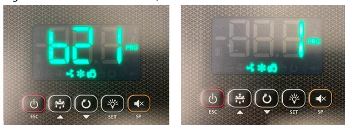
Check that all the default parameter values within the Optyma cold room control are set to site specific requirements – please note that the default alarm delay is factory set to 30 mins the high temperature alarm is set to +99°C and the low temperature alarm is set to -50 °C.
