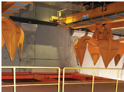
Loading crane for multiple fuel types.
