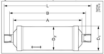
Figure 8: Solder connection (cu-plated 08-16 cu.in)
