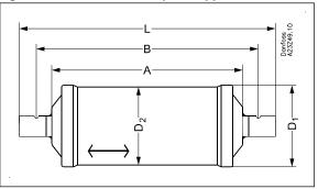
Figure 10: Solder connection (pure copper 05cu.in)
