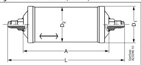
Figure 6: Flare connections (08- 16 cu.in)
