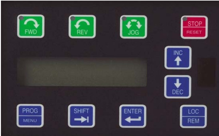
Figure 15: The Vacon 500x Keypad
