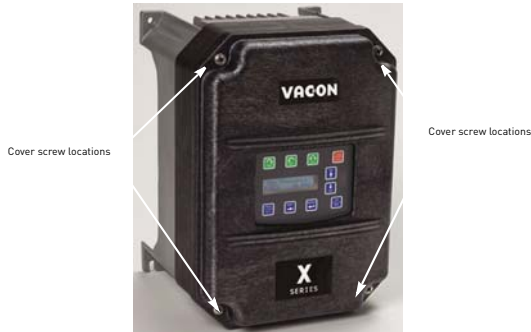
Figure 6: Vacon 500x Cover Assembly and Screw Locations
