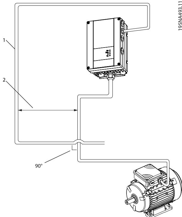
**Illustration 3.2 Minimum Distance between Communication and Power Cables**
