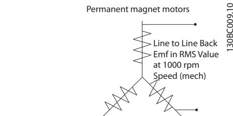
Illustration 4.3 Machine Parameter Definitions of Back EMF of PM Motors
