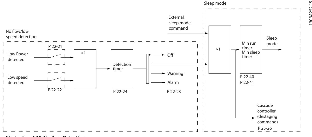
The frequency converter includes functions for detecting if the load conditions in the system allow the motor to be stopped:
