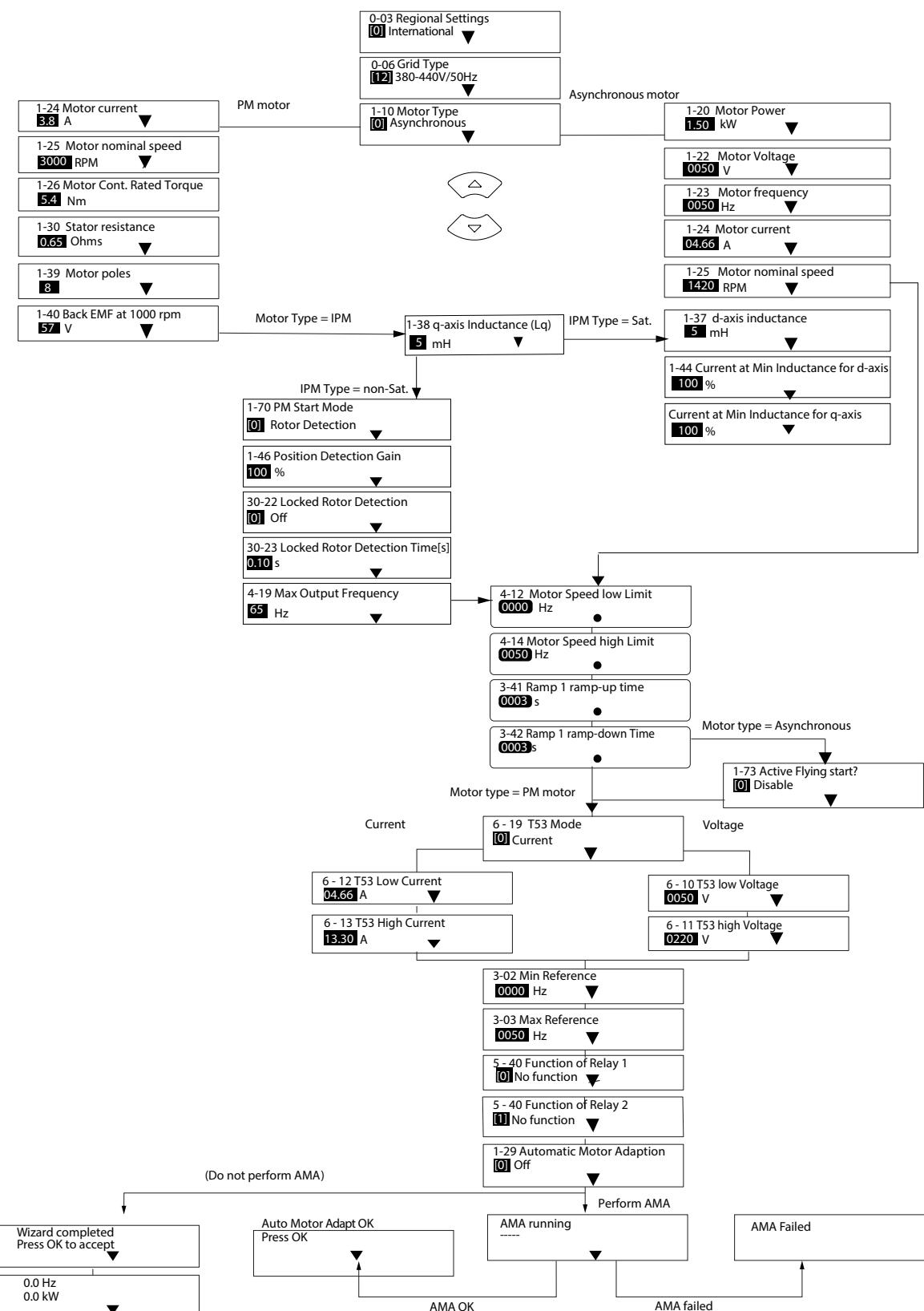
Illustration 2.3 Configuration for Open-loop Applications
