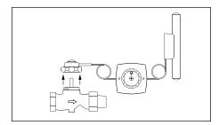
In order to use current RA 2000 operators on existing systems with Danfoss RA valves, the adapter 013G8070 must be installed to allow the new operator to fit onto the valve.
