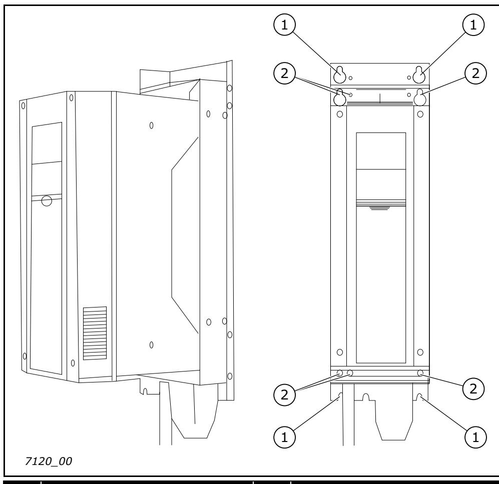
Figure 3. RFI filter back installation
