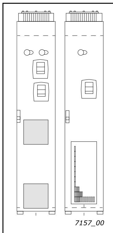
Figure 34.dU/dt filter with or without drive in enclosure
