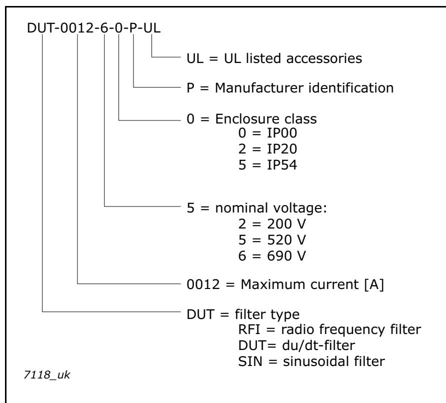
Figure 1. Type designation code for Vacon NX filters
