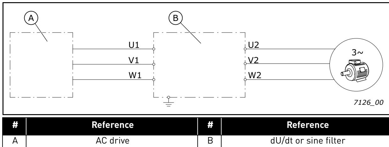
Figure 9. Filter connection
