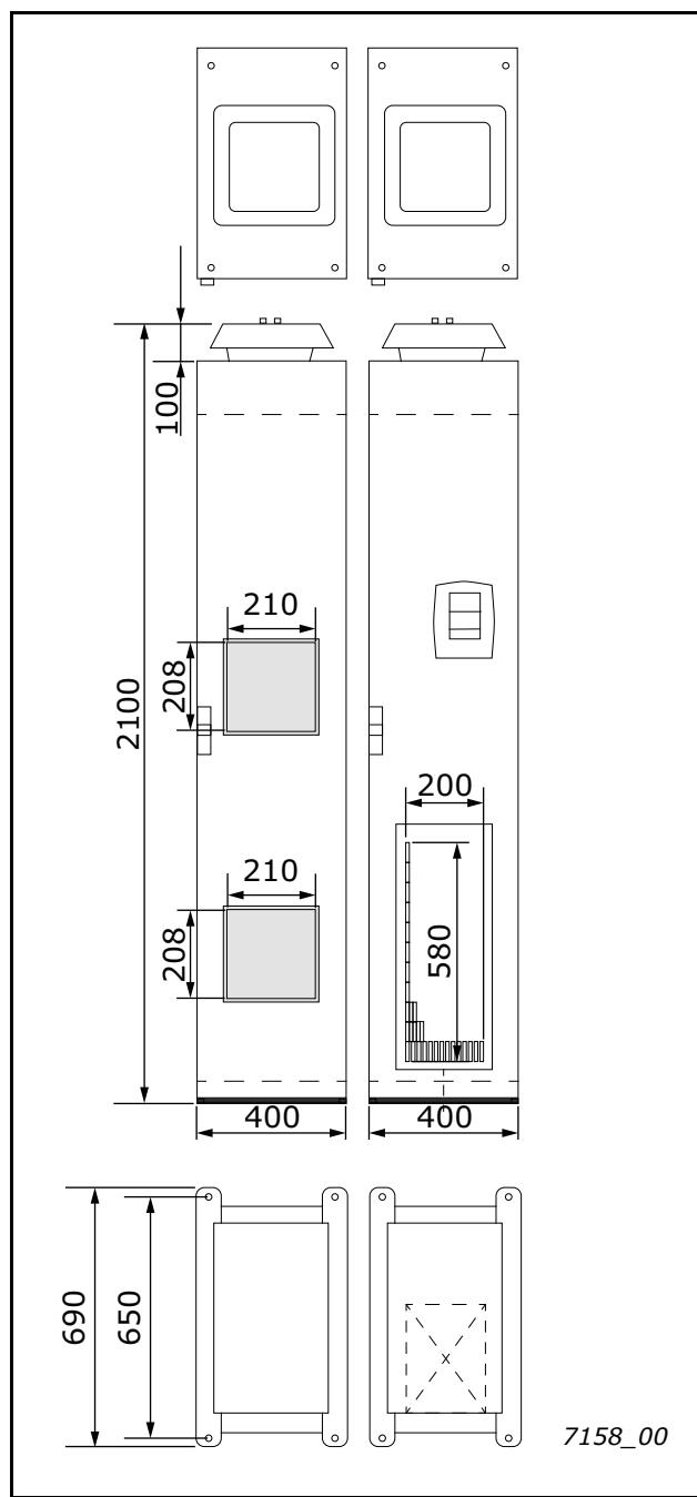
Figure 31. Chokes and dU/dt filters in enclosure
