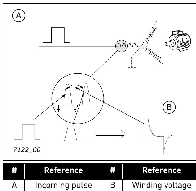
Figure 5. Change of the voltage shape in winding
