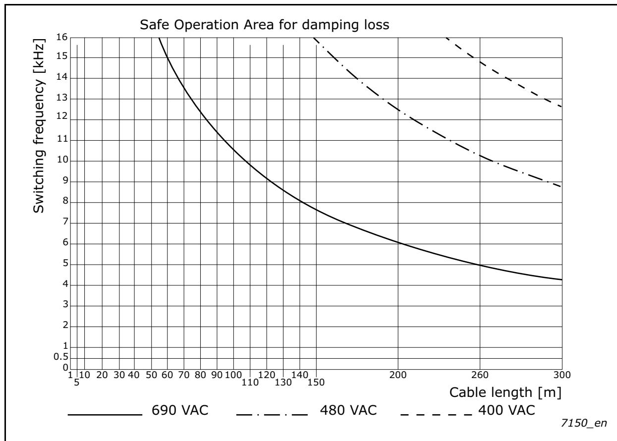
Figure 37. Safe operating area for DUT 0420 6 0 S
