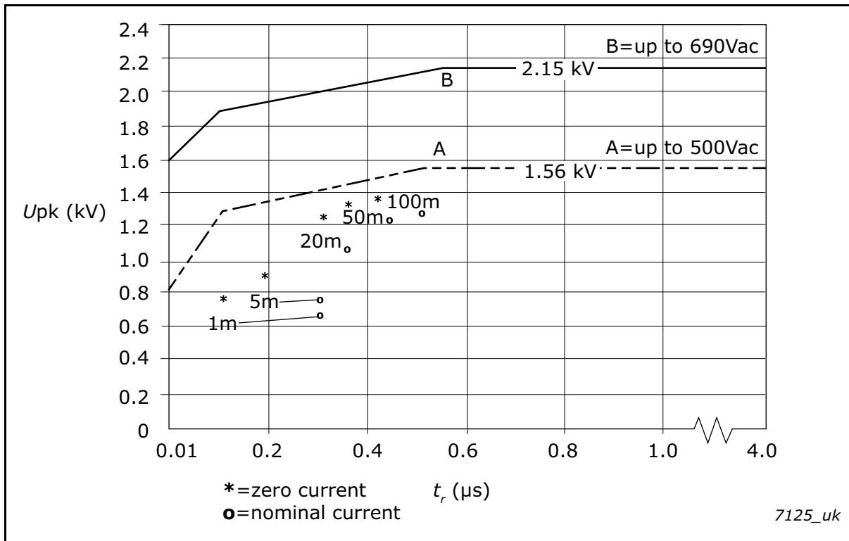
Figure 8. IEC/TC60034-25: Limiting curves of impulse voltage  $U_{pk}$ , measured between two motor phase terminals, as a function of the peak rise time  $t_r$ . Typical values achieved with Vacon AC drives.
