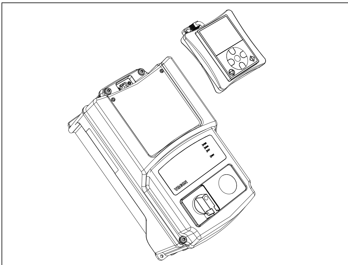
Figure 48. Mounting of the keypad.
