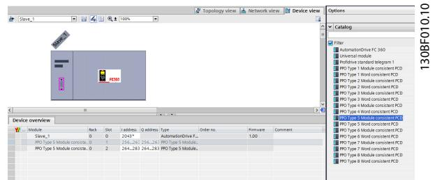
**Illustration 3.7 Drag and Drop PPO Type 6 Word Consistent to the First Slot**
