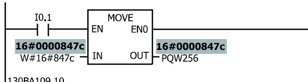
**Illustration 7.6 Network Reverses the Motor When Digital Input 19 is ON**
