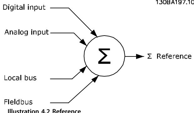
The reference, or speed setpoint, is sent via PROFIBUS and is always transmitted to the frequency converter in percentage format as integers shown in hexadecimal (0–4000 hex).
