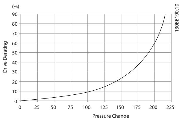
**Illustration 3.19** Enclosure Size F, Derating vs. Pressure Change (Pa)Drive air flow: 985 m<sup>3</sup>/h (580 cfm)
