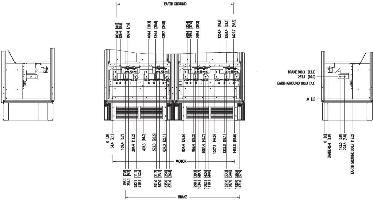
Illustration 3.14 Terminal Locations - Left, Front and Right Views. The gland plate is 42 mm below .0 level.
