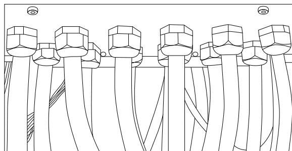
**Illustration 3.20** Example of Proper Installation of the Gland Plate.
