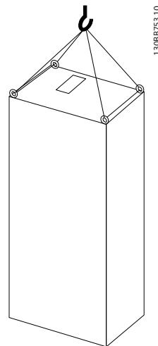
Illustration 3.1 Recommended Lifting Method, Enclosure Size F8.
