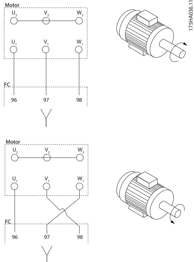
Illustration 4.13 Wiring for Clockwise and Counterclockwise Motor Rotation
