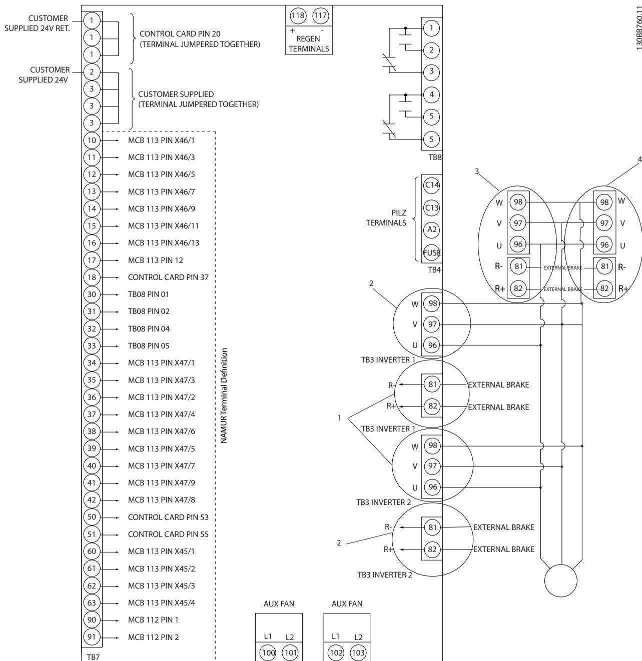
**Illustration 4.25 Diagram Showing all Electrical Terminals with NAMUR Option**
