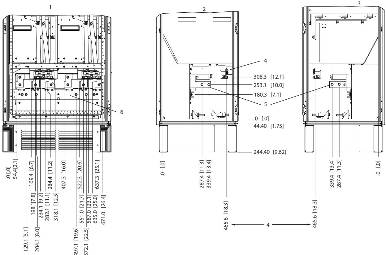
Illustration 3.12 Terminal Locations - Left, Front and Right Views. The gland plate is 42 mm below .0 level.
