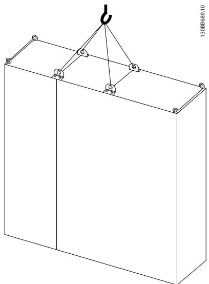
Illustration 3.3 Recommended Lifting Method, Enclosure Size F11/F12/F13/F14.
