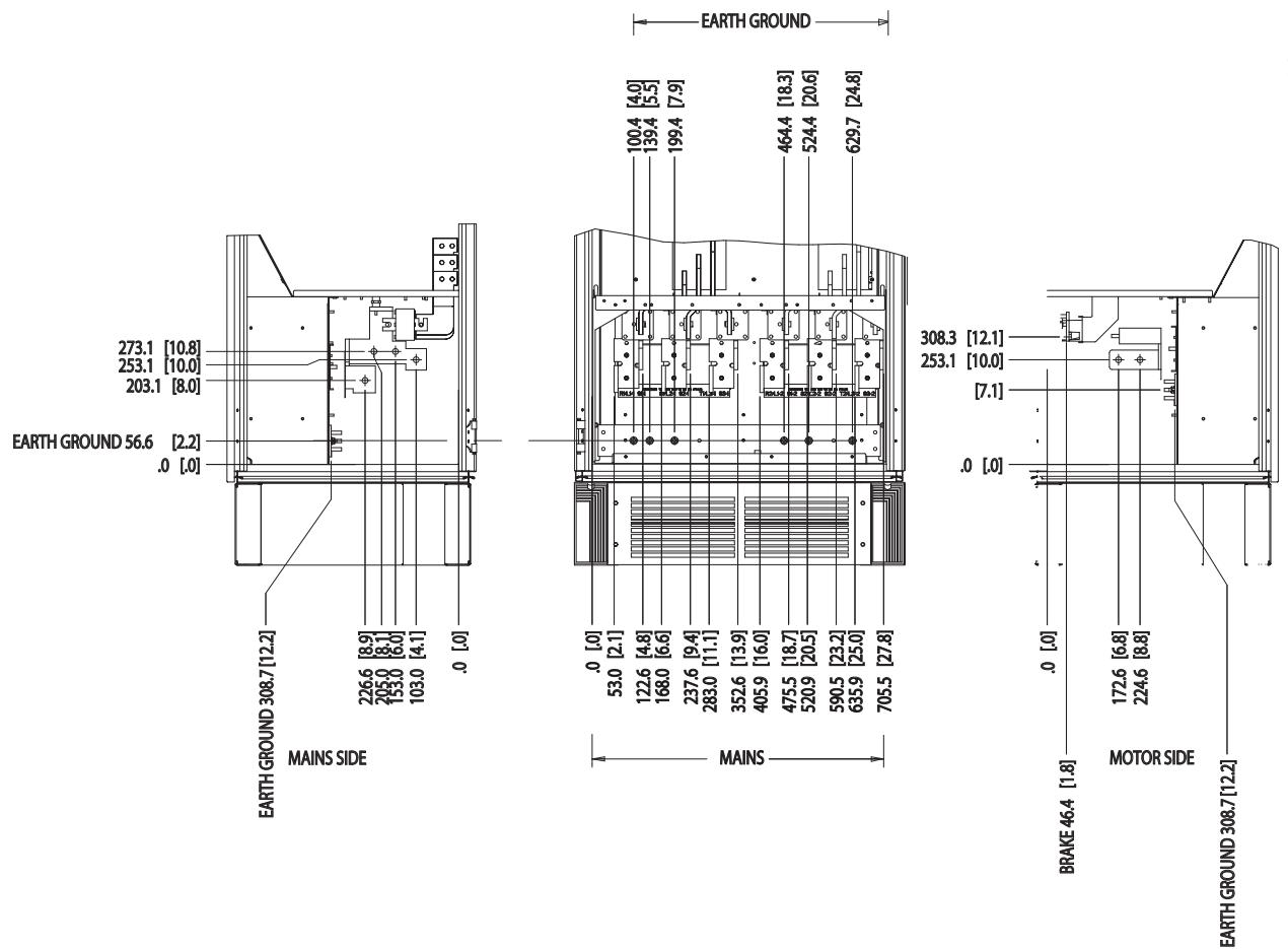
Illustration 3.16 Terminal Locations - Left, Front and Right Views. The gland plate is 42 mm below .0 level.
