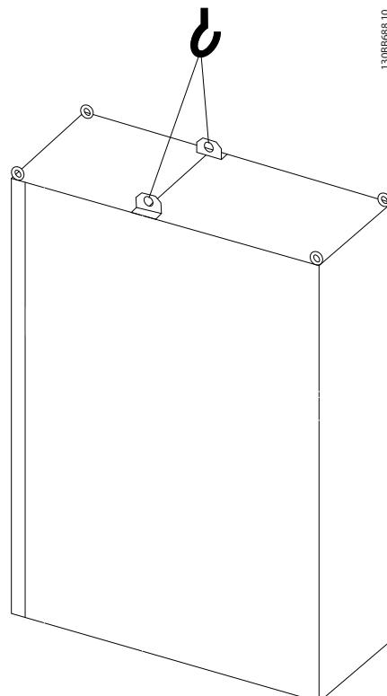
Illustration 3.2 Recommended Lifting Method, Enclosure Size F9/F10.
