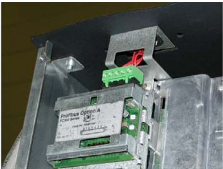
Figure 4.17: Top connection for serial communication bus.
