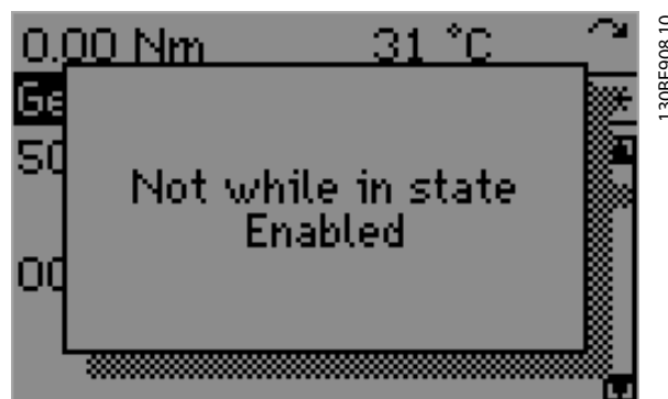
Illustration 4.25 Rejection of Hand On Mode on a Servo Drive while in State Operation enabled
