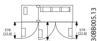
Illustration 3.13 Space in Front of IP21/IP54 Rated Enclosure Type F2
