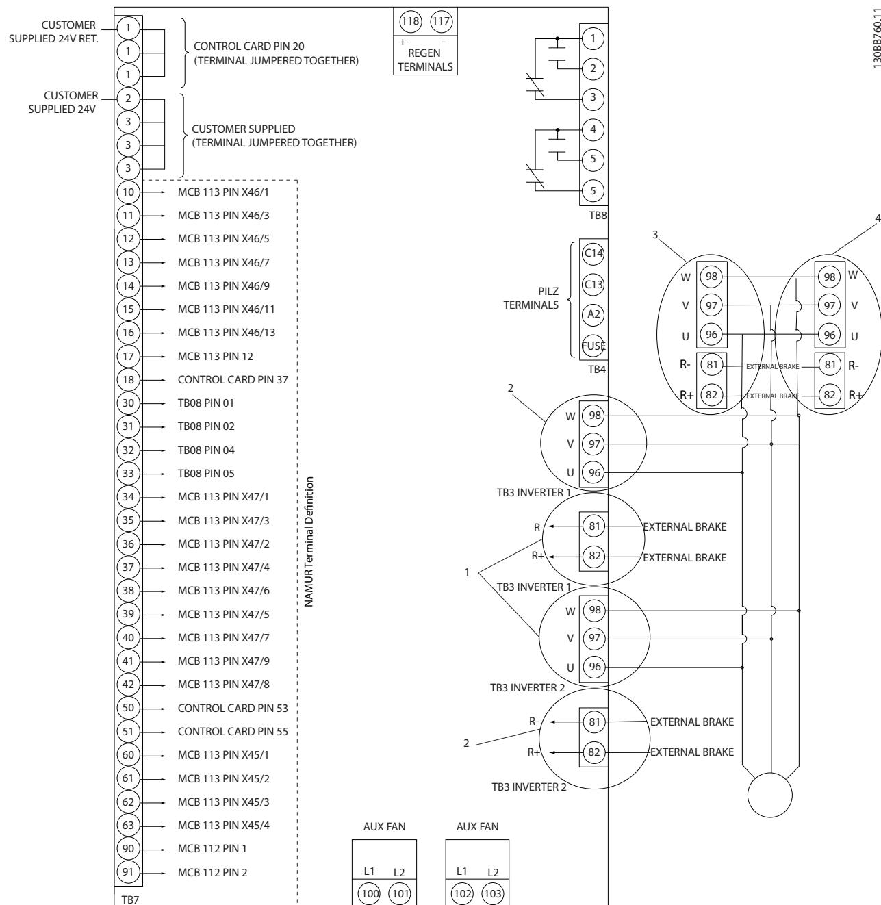
**Illustration 3.75 Diagram Showing all Electrical Terminals with NAMUR Option shown in Dotted Line Box**
