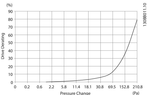
Illustration 3.33 E frame Derating vs. Pressure Change (Large Fan), P315T5-P400T5 and P500T7-P560T7
