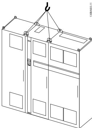
**Illustration 3.4 Recommended Lifting Method, Enclosure Type F3 (460 V, 600 to 900 HP, 575/690 V, 900 to 1150 HP)**
