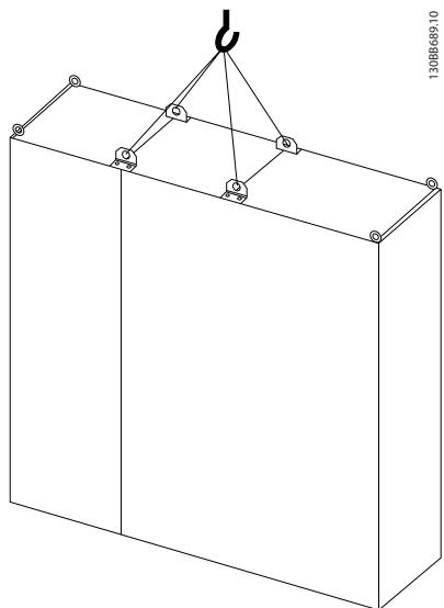
Illustration 3.8 Recommended lifting method, Enclosure Type
