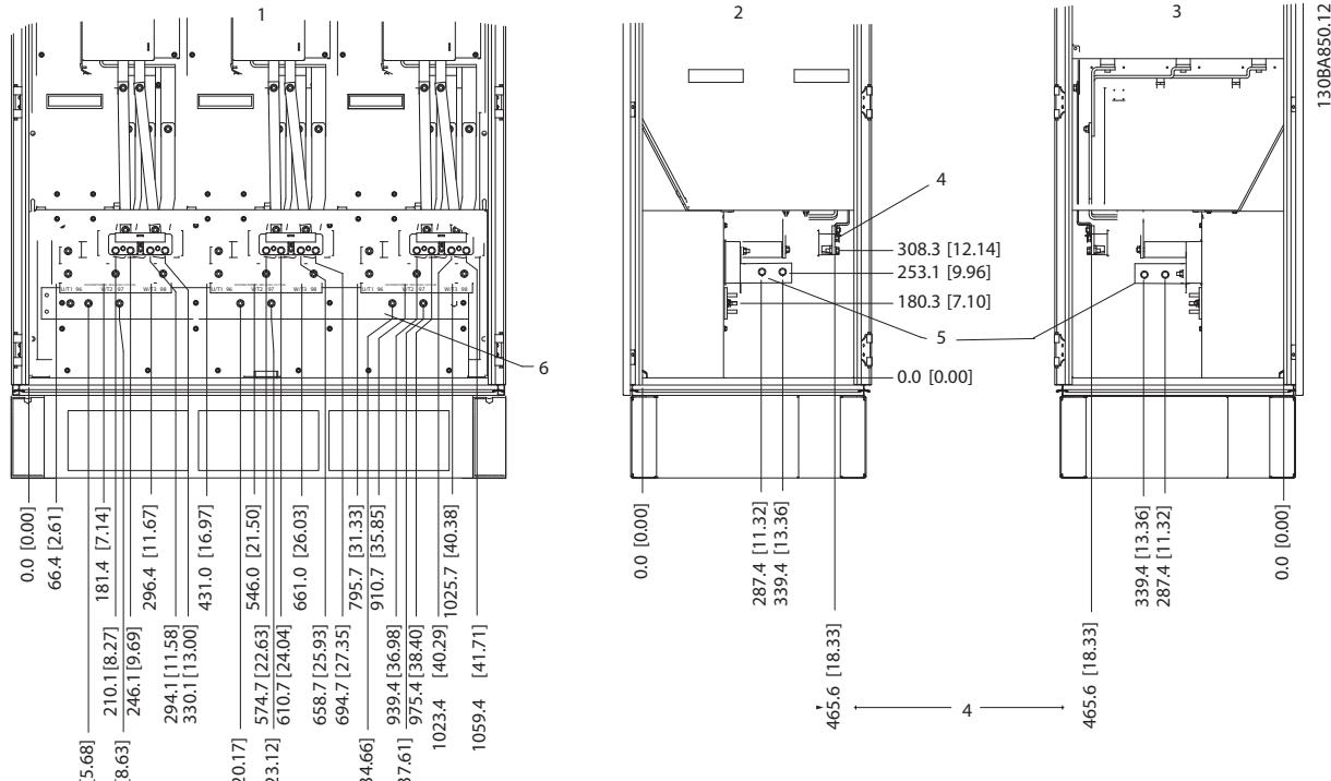
**Illustration 3.26 Terminal locations - Inverter Cabinet - F2 and F4 (front, left and right side view). The gland plate is 42 mm below .0 level.**
