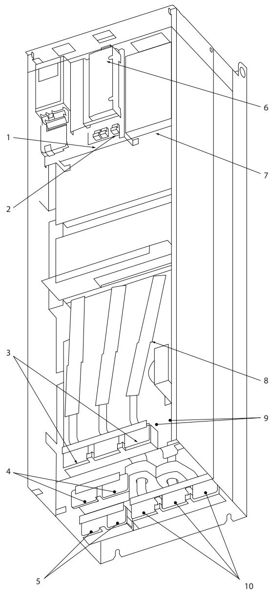
Illustration 3.52 Compact IP00 (Chassis), Enclosure Type D3
