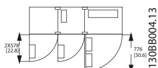
Illustration 3.12 Space in Front of IP21/IP54 Rated Enclosure Type F3
