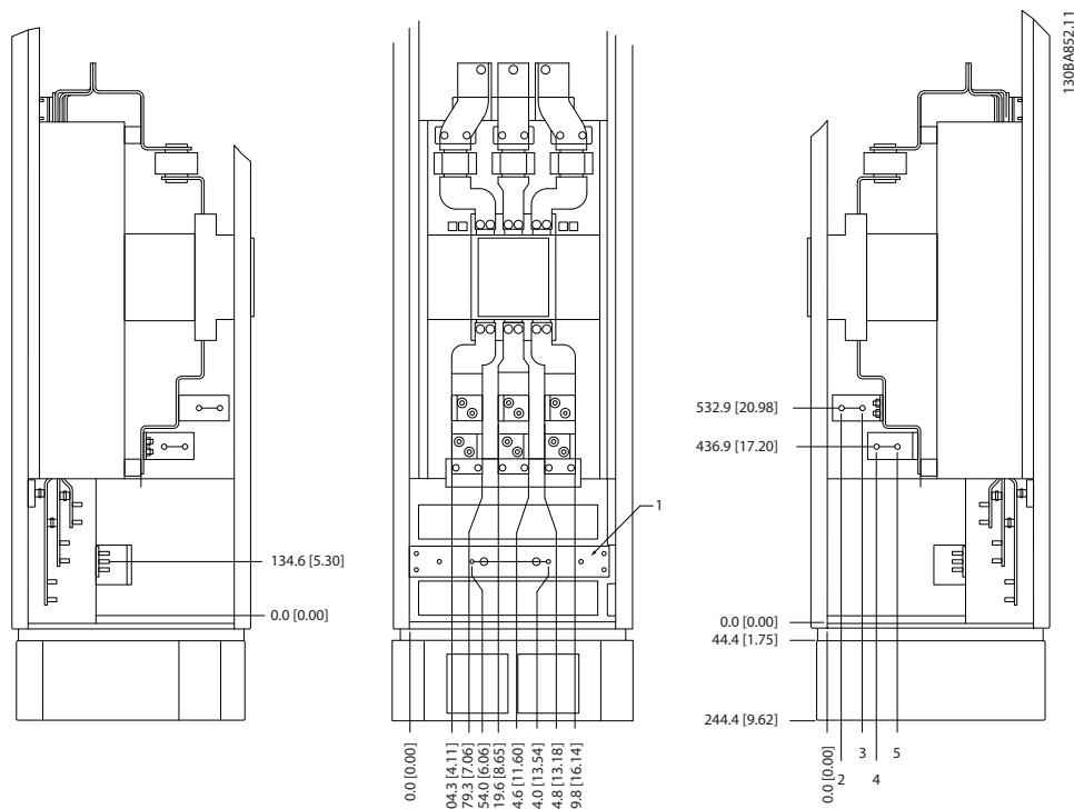
Illustration 3.30 Terminal locations - Options Cabinet with circuit breaker/ molded case switch (Left side, front and right side view).
