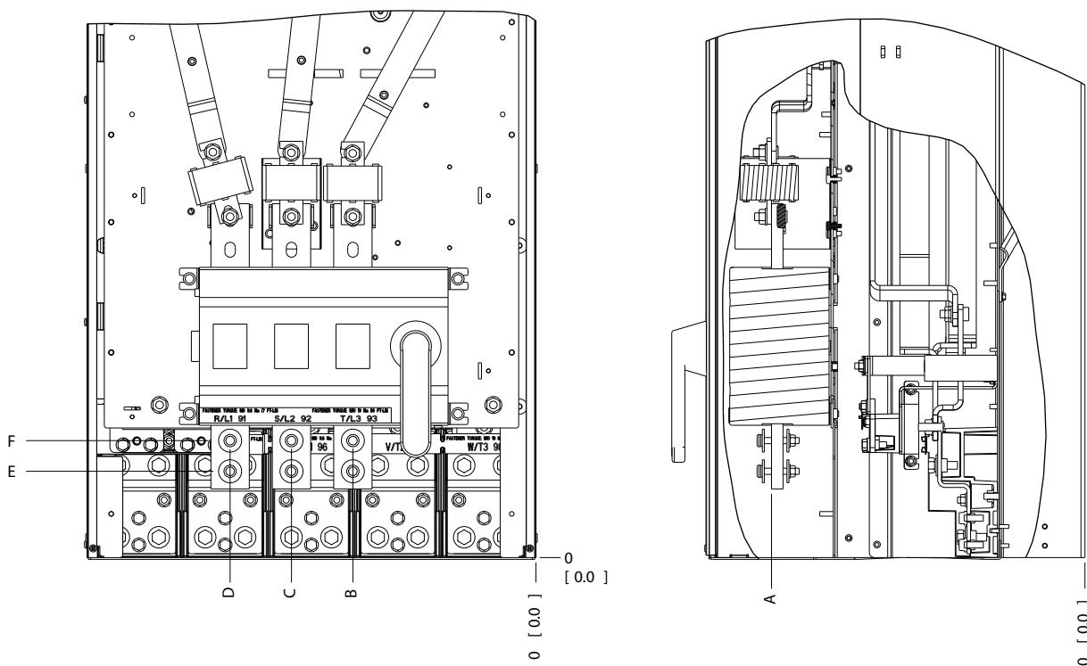
Illustration 3.22 IP00 Enclosure Power Connections Positions of Disconnect Switch
