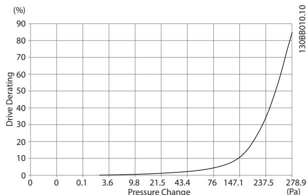
Illustration 3.32 E frame Derating vs. Pressure Change (Small Fan), P250T5 and P355T7-P400T7
