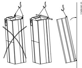
Illustration 3.1 Recommended Lifting Method, Enclosure Types D and E
