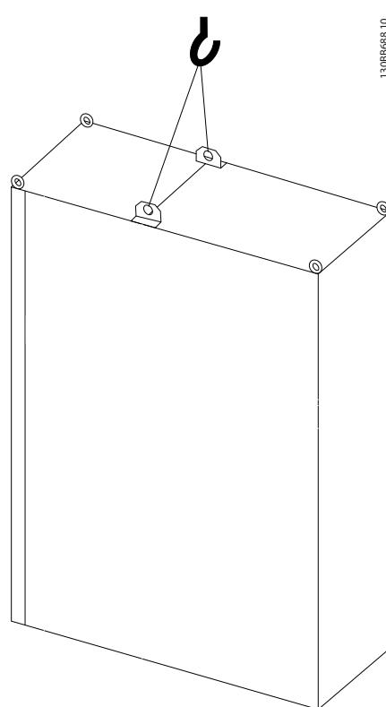
**Illustration 3.7 Recommended lifting method, Enclosure Type F9/F10**
