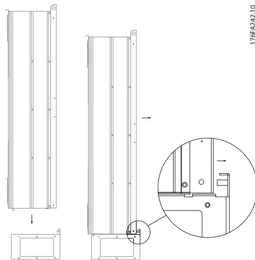
Illustration 3.47 Mounting of Frequency Converter to Pedestal
