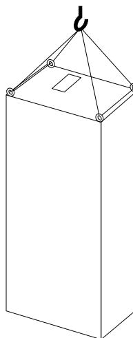
**Illustration 3.6 Recommended lifting method, Enclosure Type F8**
