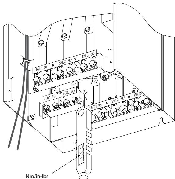
Illustration 3.63 Tightening Bolts with a Torque Wrench
