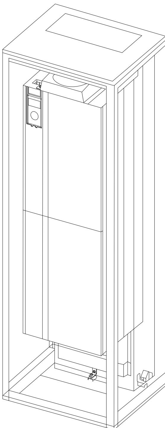
Illustration 3.44 Installation of IP00 in Rittal TS8 Enclosure.
