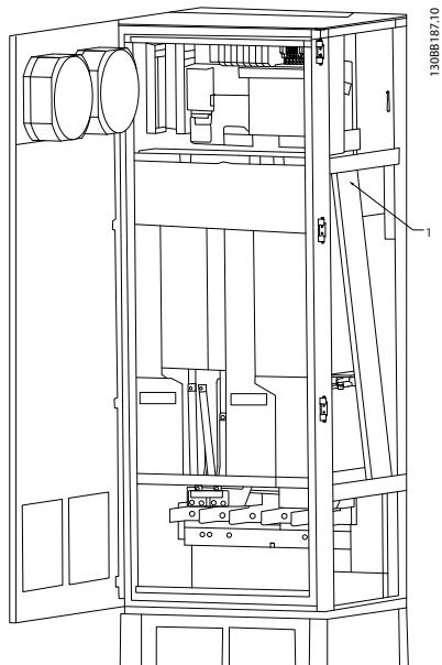
**Illustration 3.66 Control Card Wiring Path for the F1/F3.** Control Card Wiring for the F2/F4 use the same Path
