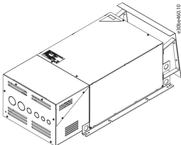
Illustration 7.39 IP21 X3-V3 Internal and Internal Fan, 3D View
