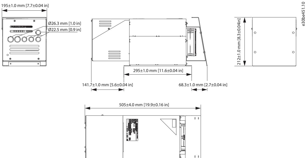
Illustration 7.34 IP21 X1-V3 Internal and External Fan
