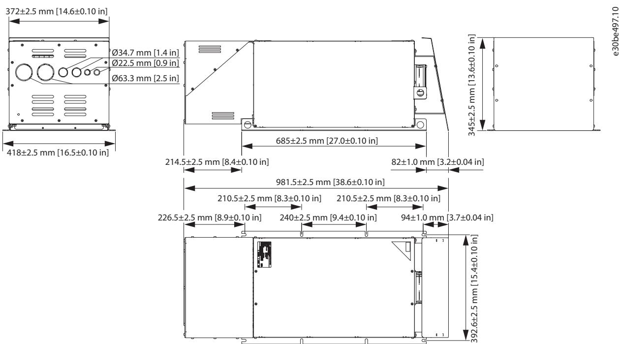
**Illustration 7.42 IP21 X5-V3 Internal and External Fan**
