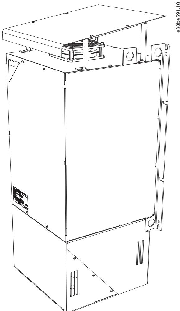
**Illustration 5.1 IP21/NEMA 1 Kit, Internal Fan and External Fan**
