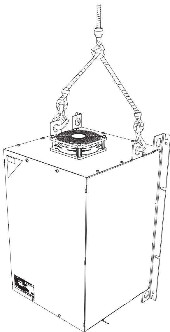
Illustration 4.2 Recommended Lifting Method, External Fan Filters
