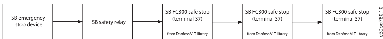
Illustration 5.8 Safety-related Block Diagram
