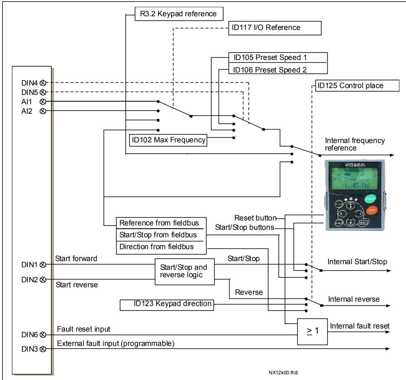
Figure 7. Control signal logic of the Basic Application
