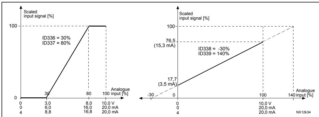
Figure 36. Examples of actual value signal scaling
