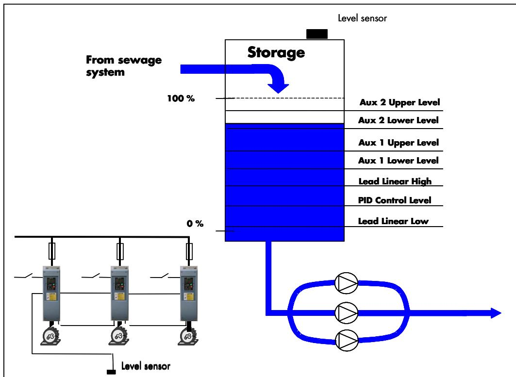
Figure 12. Principle of Advanced Level Control system
