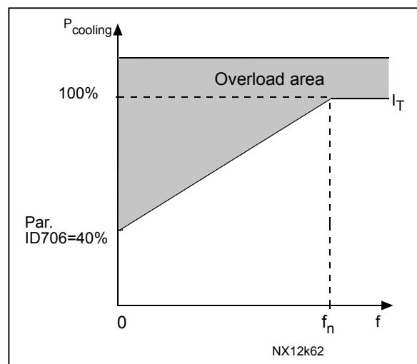
Figure 42. Motor thermal current  $I_T$  curve
