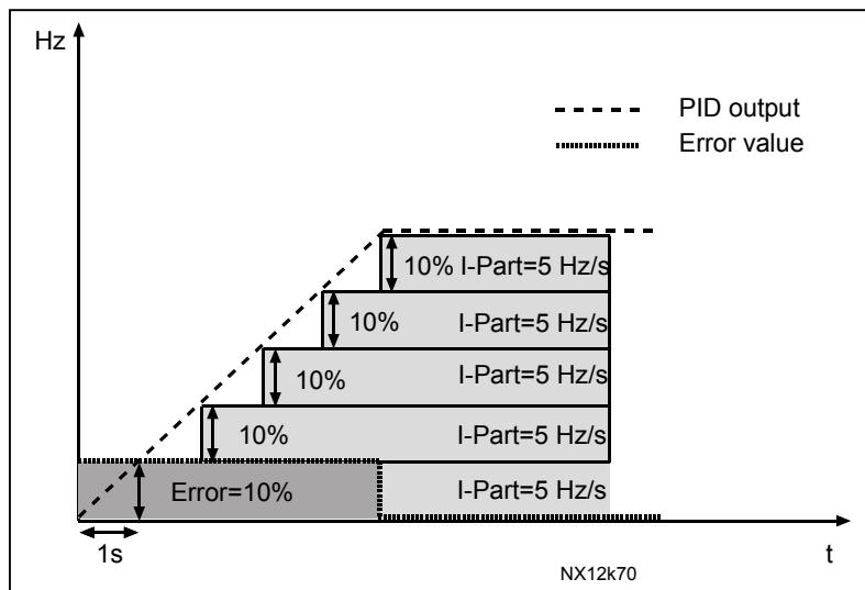
Figure 24. PID controller function as I-controller.
