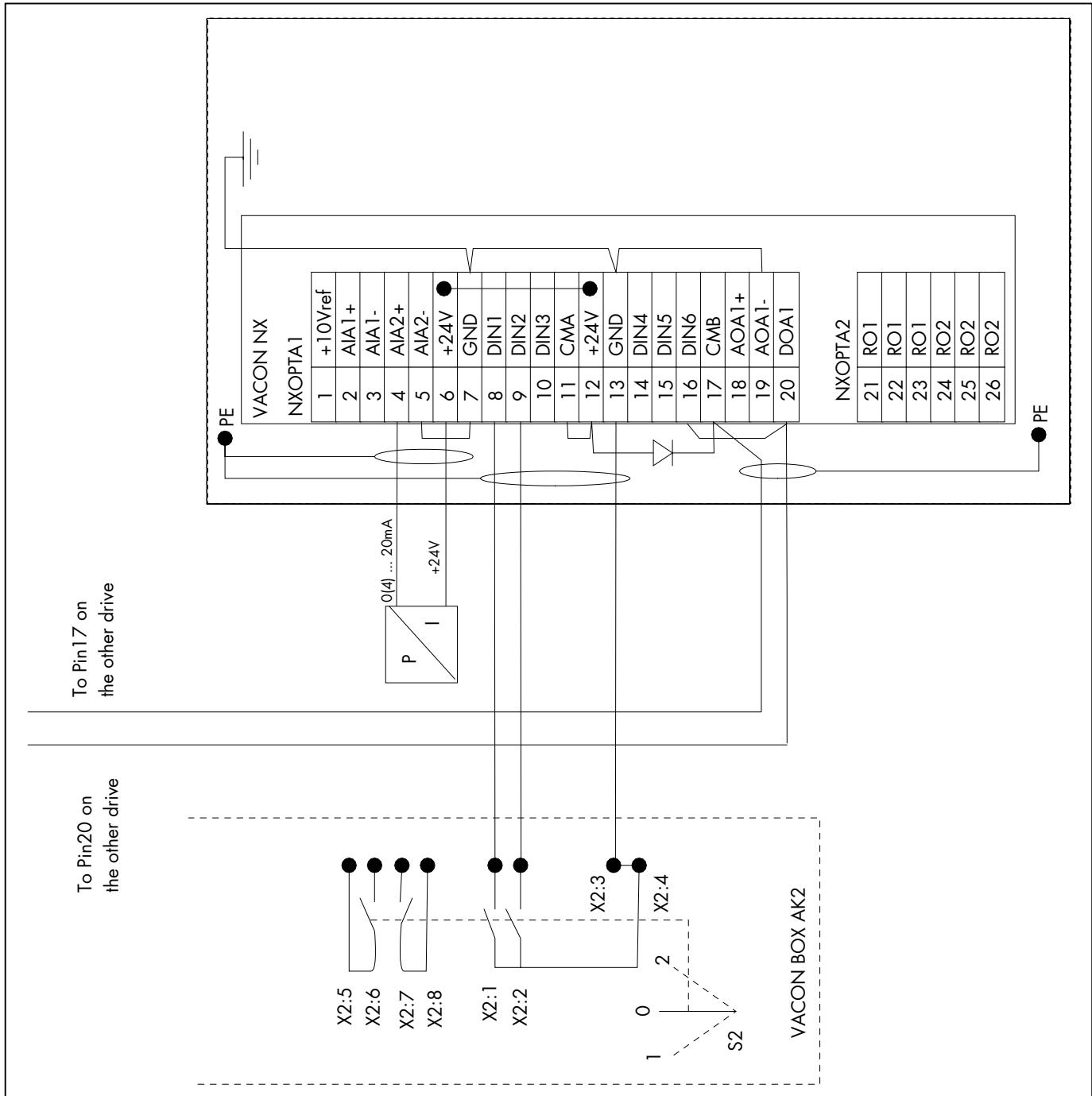
Figure 6. Advanced Level Control Application, control diagram
