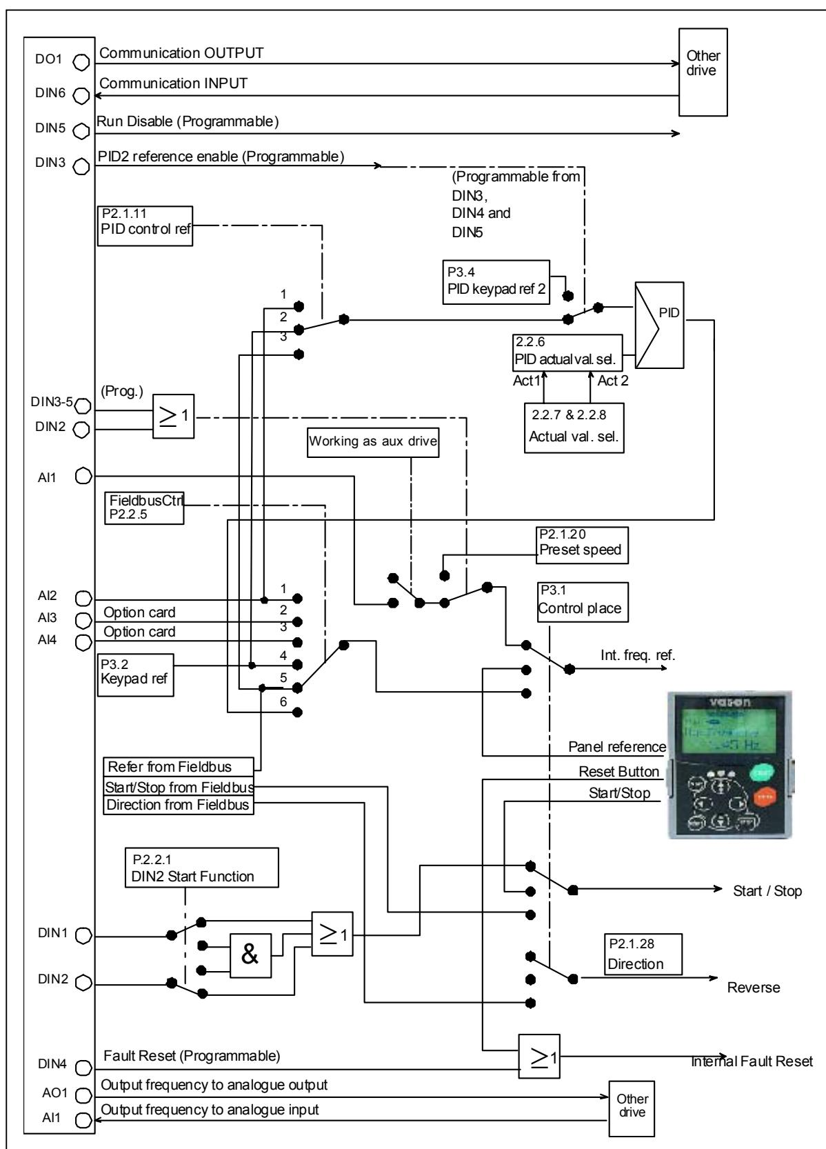
Figure 21. Control I/O logic, MultiFollower PFC Application
