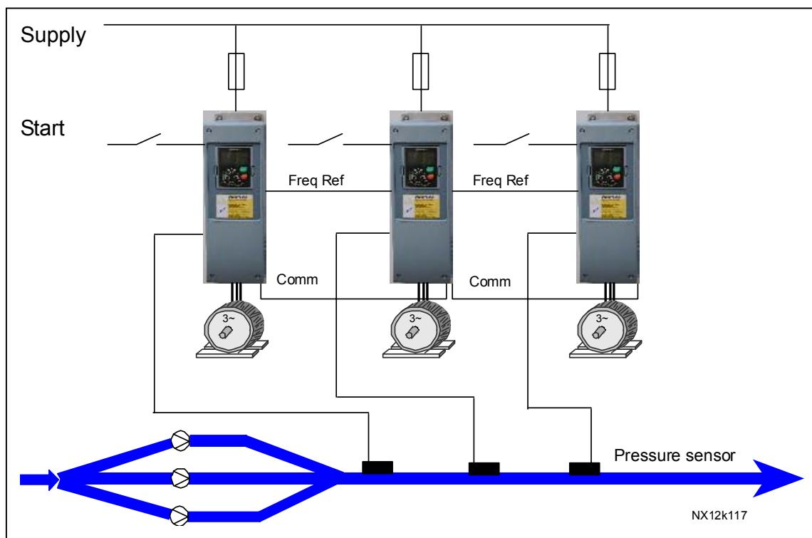
Figure 16. Operating principle of MultiFollower PFC system
