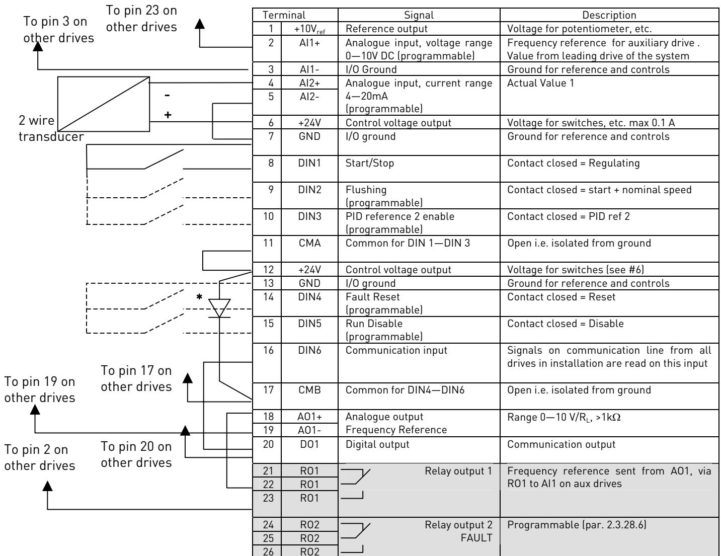
Figure 19. I/O configuration for the MultiFollower PFC Application
