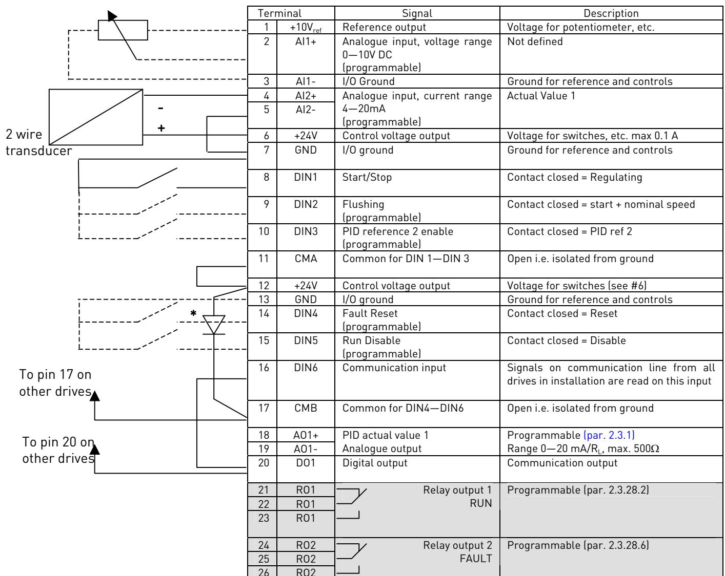
Figure 13. I/O configuration for the MultiMaster PFC application
