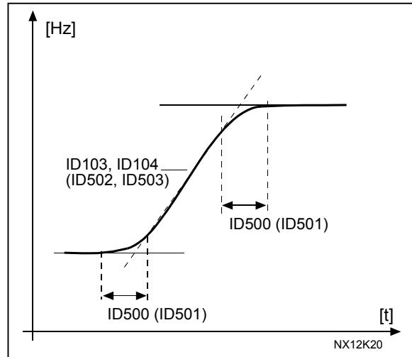
Figure 37. Acceleration/Deceleration (S-shaped)
