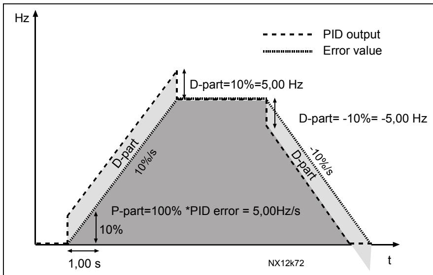
Figure 26. PID output with the values of Example 3.
