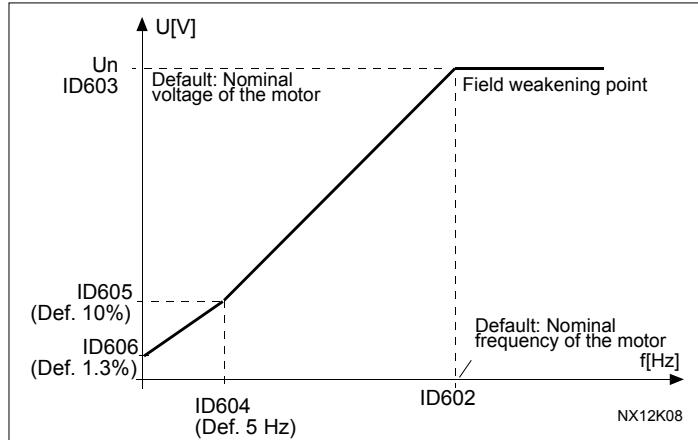
Figure 23. Programmable U/f curve
