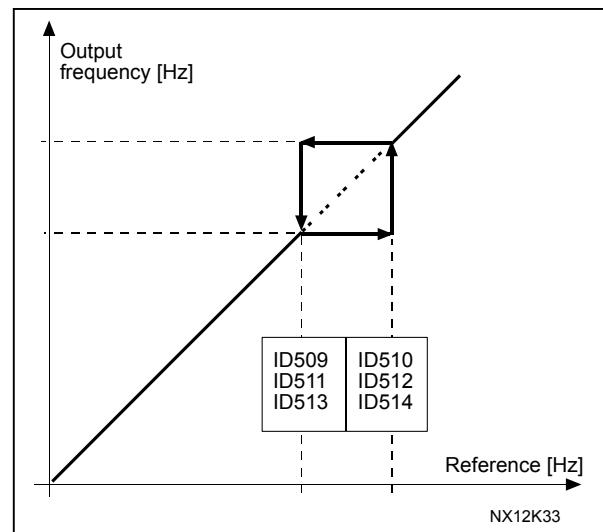
Figure 40. Example of prohibit frequency area setting.
