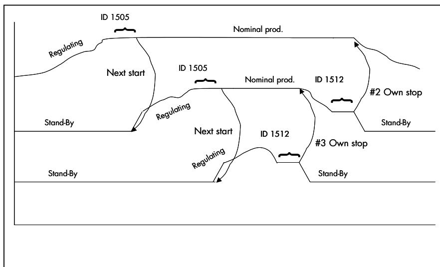
Figure 51. Use of parameters ID1505 and ID1512
