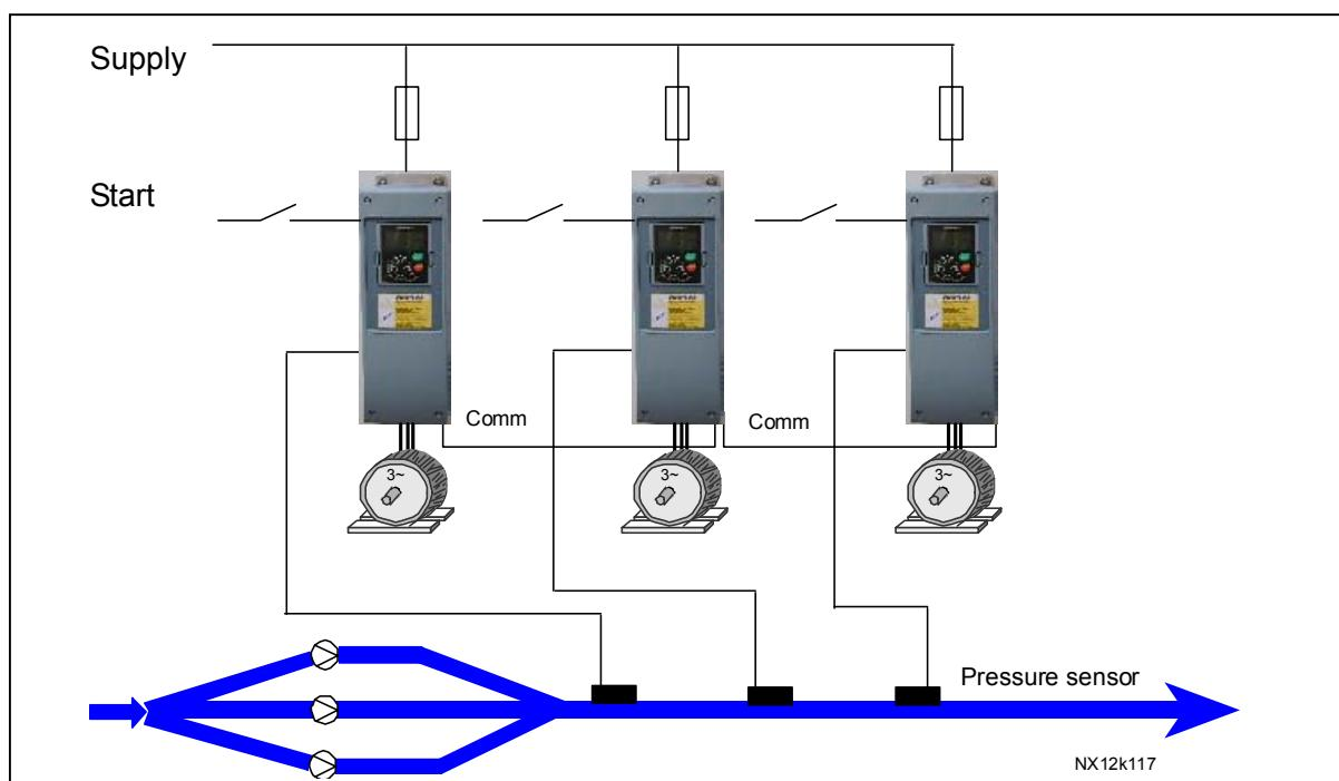
Figure 8. Operating principle of MultiMaster PFC system
