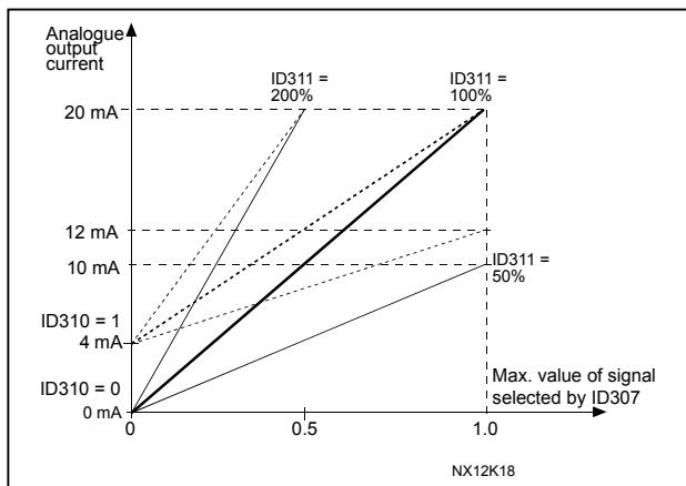
Figure 30. Analogue output scaling
