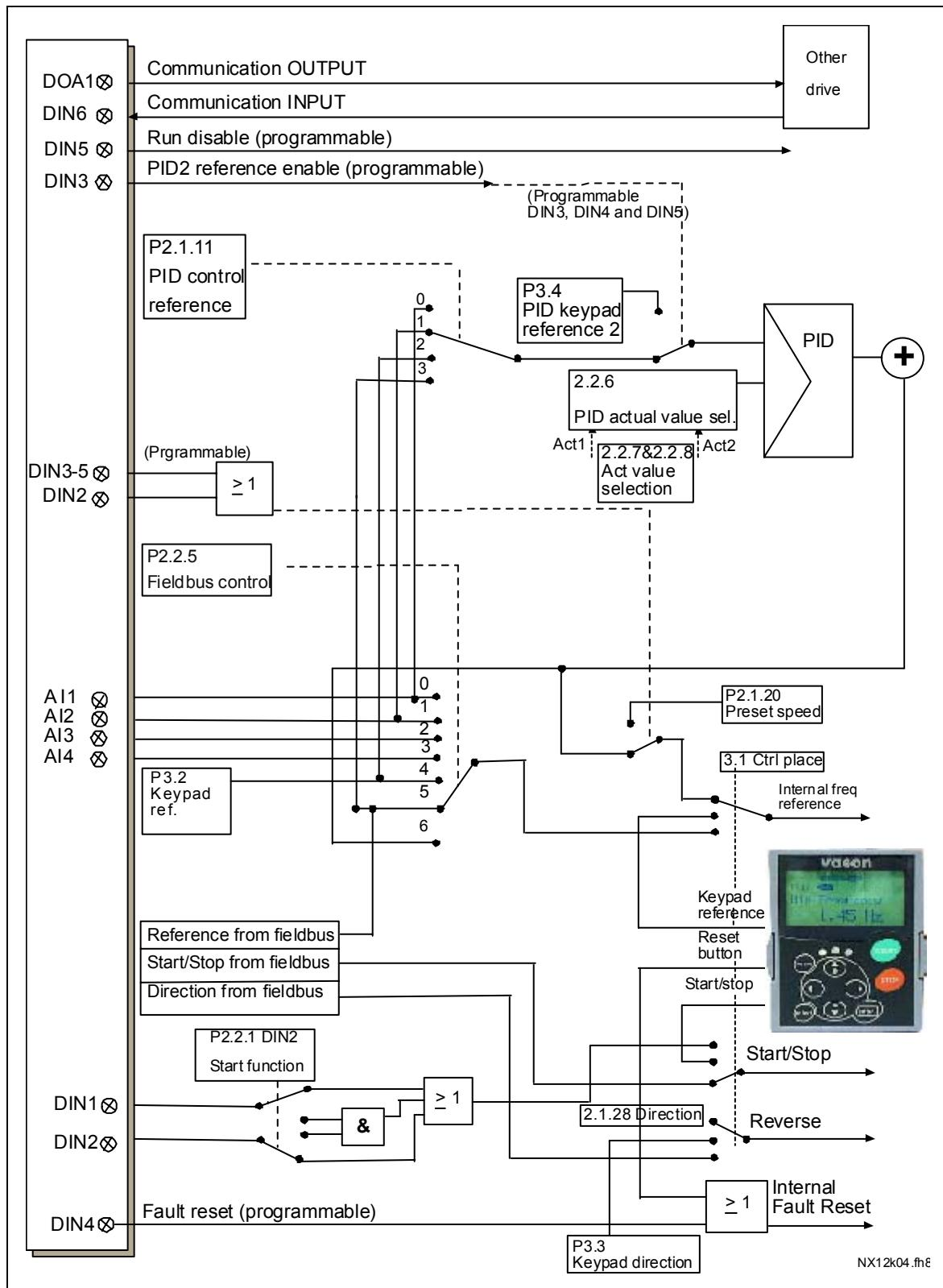
Figure 11. Control signal logic in MultiMaster PFC Application
