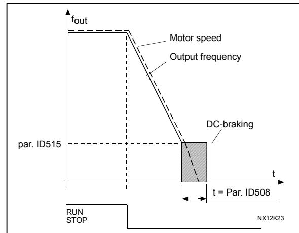
Figure 39. DC-braking time when Stop mode = Ramp
