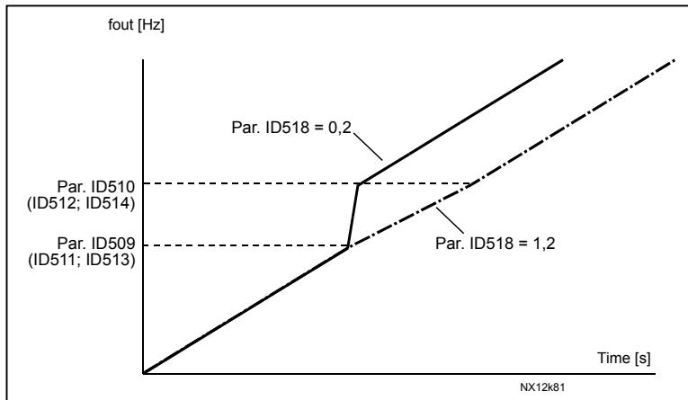
Figure 41. Ramp speed scaling between prohibit frequencies
