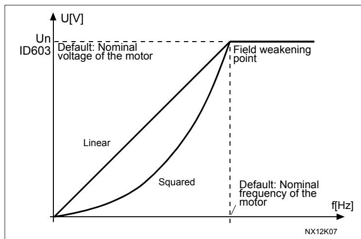
Figure 22. Linear and squared change of motor voltage
