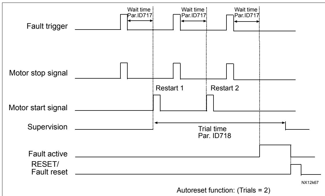
*Figure 48. Example of Automatic restarts with two restarts*
