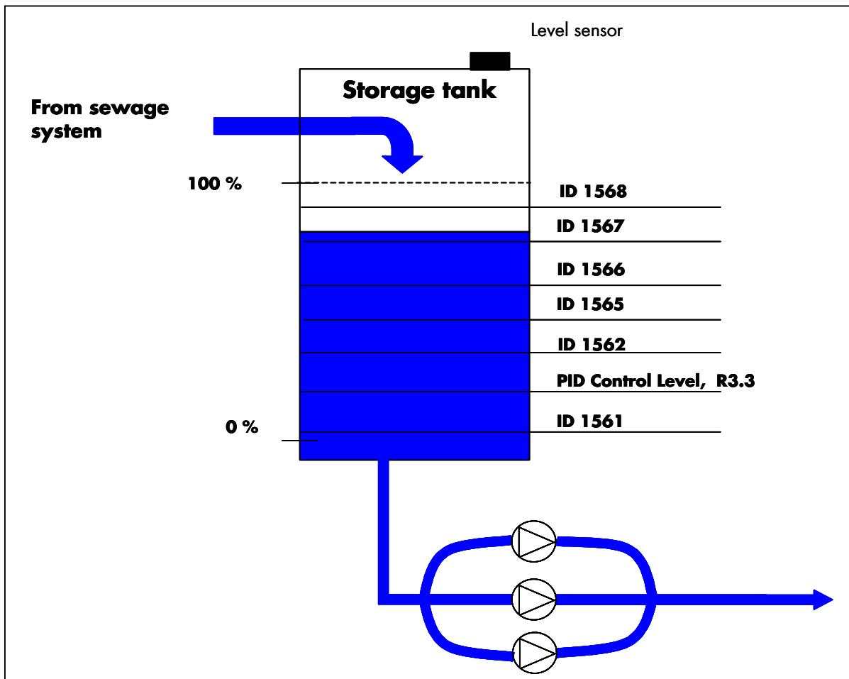
Figure 53. Different levels in Advanced Level Control application
