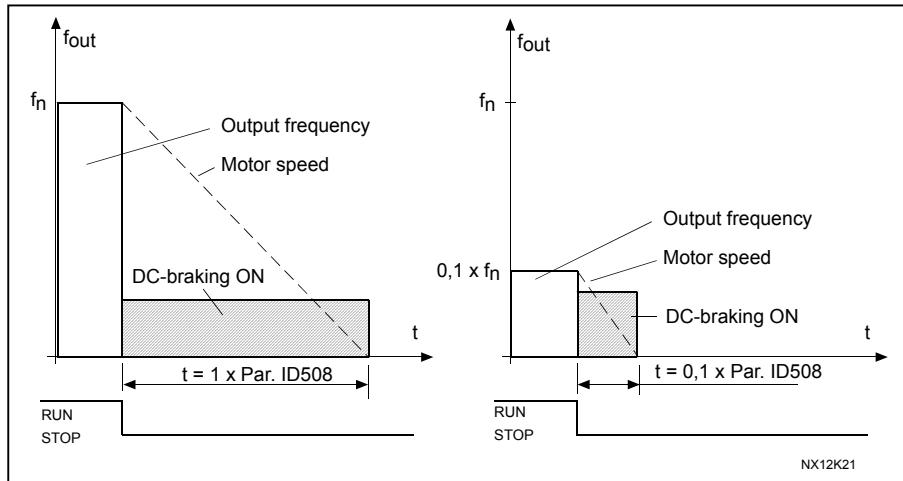
Figure 38. DC-braking time when Stop mode = Coasting.
