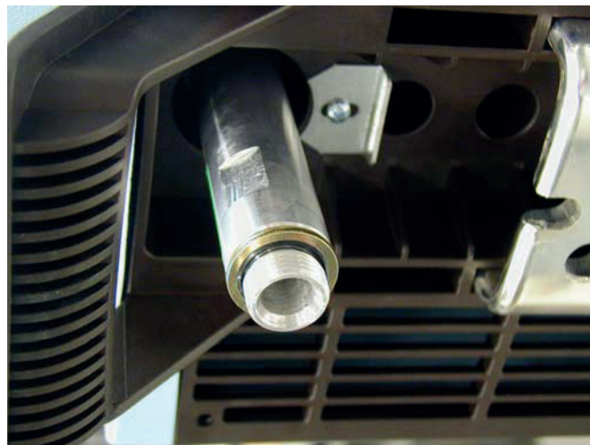
Figure 28. External thread of hose adapter
