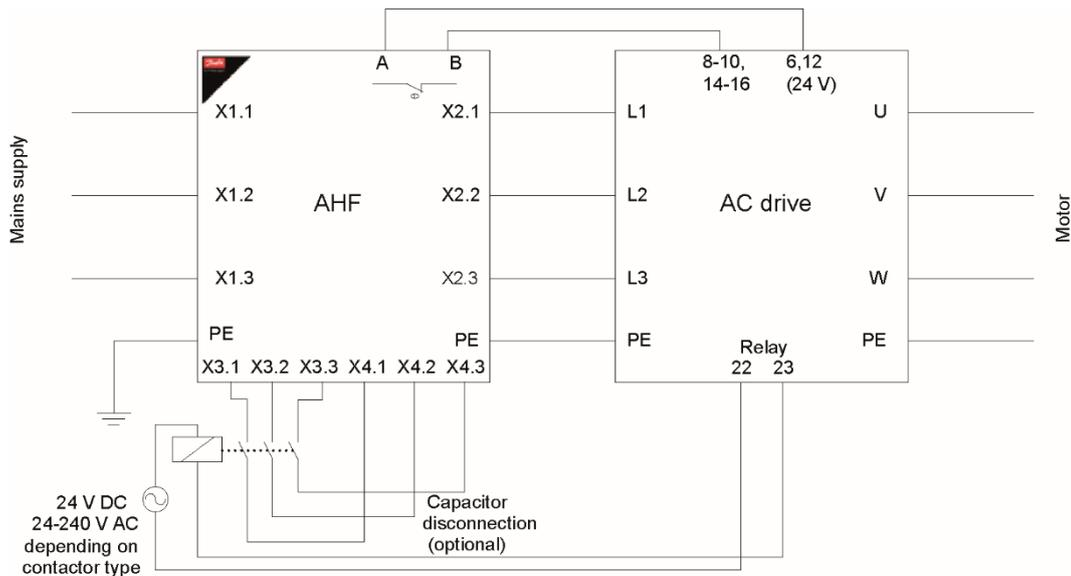
Figure 1. Connection diagram with VACON® 100 Family terminals
