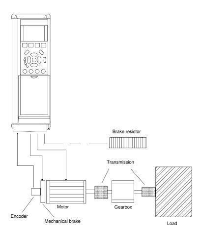
Illustration 40: Basic Set-up for Closed-loop Speed Control
