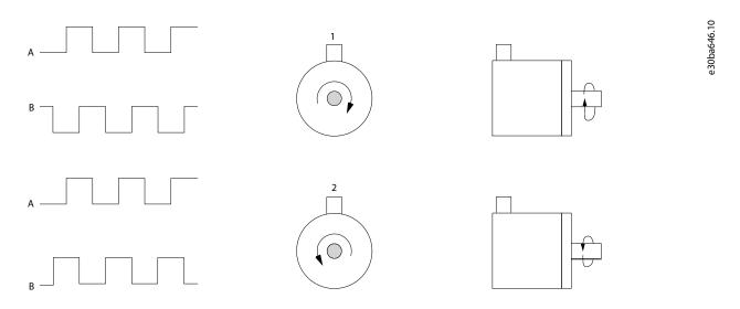
Illustration 45: Determining Encoder Direction
