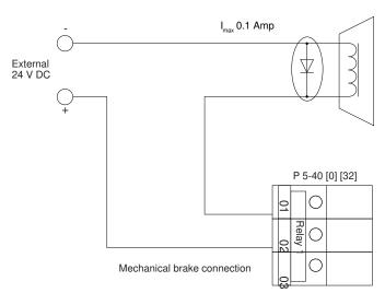
Illustration 47: Wire Configuration for Torque and Stop Limit
