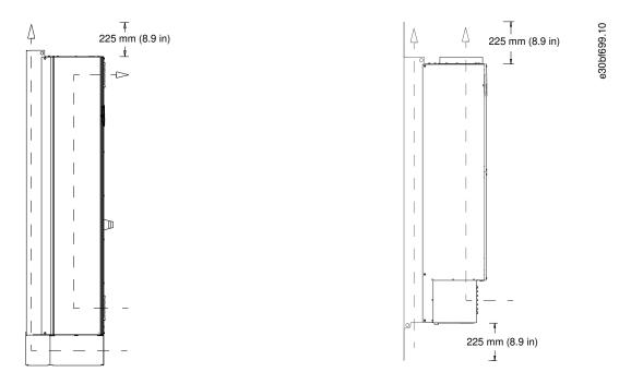
Illustration 69: Airflow for E1h/E2h (Left) and E3h/E4h (Right)
