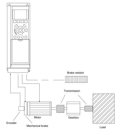
Illustration 40: Basic Set-up for Closed-loop Speed Control
