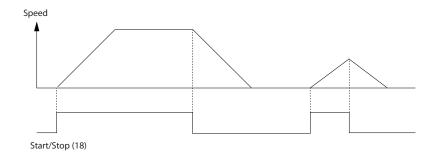
Illustration 42: Start/Stop Command with Safe Torque Off
