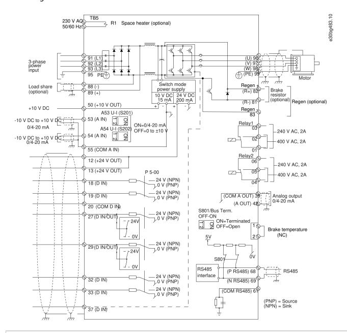
1 Terminal 37 (optional) is used for Safe Torque Off. Refer to the VLT® FC Series - Safe Torque Off Operating Guide for installation instructions.
