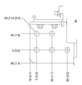
Illustration 27: E3h Mains, Motor, and Ground Terminal Dimensions (Side Views)
