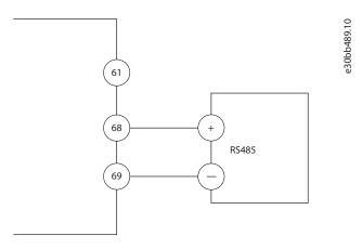
Illustration 38: Serial Communication Wiring Diagram
