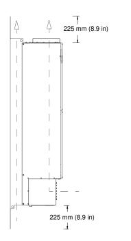
Illustration 69: Airflow for E1h/E2h (Left) and E3h/E4h (Right)
