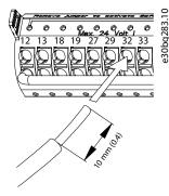
Illustration 36: Connecting a Solid Control Cable to the Terminal Box
