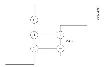
Illustration 38: Serial Communication Wiring Diagram
