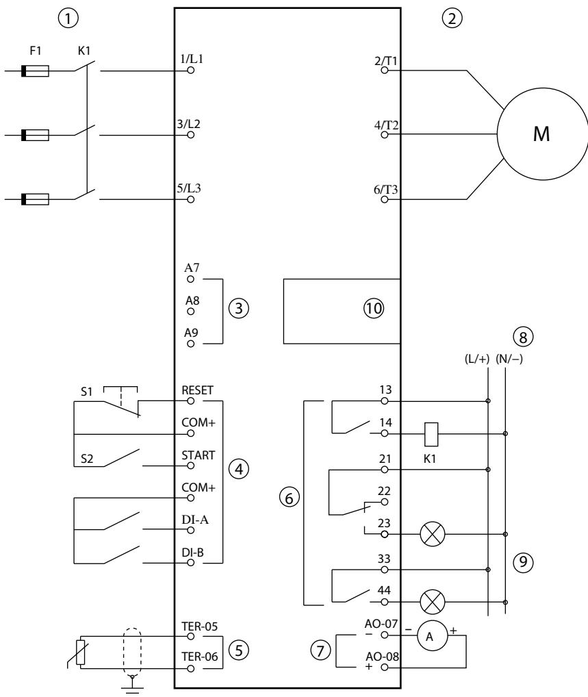
Externally bypassed/Externem Bypass/Bypass externe/Bypass esterno/Bypass externo/Bypass externo/外部旁路安装示例
