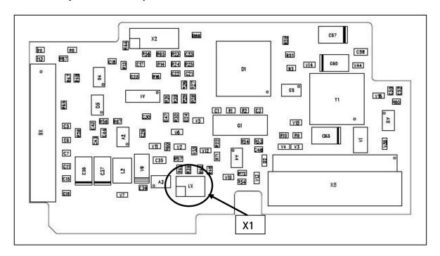
Description: Encoder board for VACON® NXP with an input for Sin/Cos type encoder.
