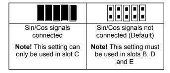
**NOTE!** Be careful with the jumper settings, wrong settings may damage the encoder.
