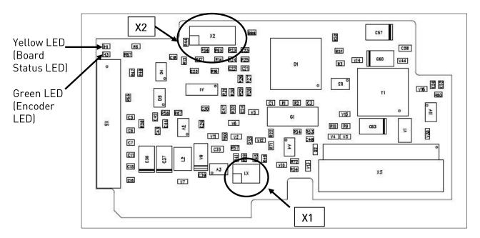
Description: Encoder board for VACON® NXP with an input for EnDat/SSI absolute encoder
