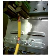
Make a sufficiently wide opening for your cable by cutting the grid as wide as necessary.
