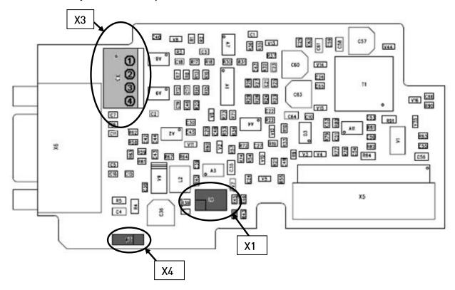
Description: Encoder board for VACON® NXP with an input for Sin/Cos type encoder.
